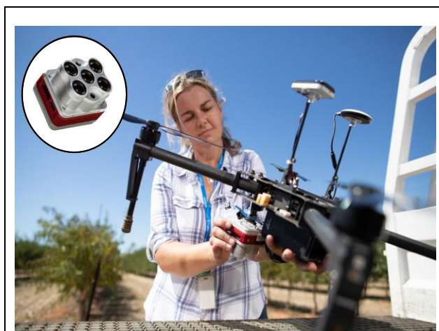
Figure 38 An Altum multispectral camera being connected to the DJI Matrice 100 with the Altum Skyport connection.
