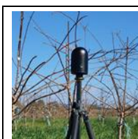
Figure 37 LiDAR unit used to scan trees
