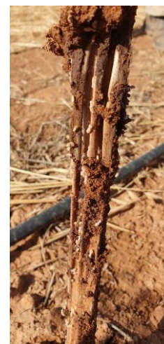
Figure 31 Termite damage on hardwood stakes in the H1 planting
