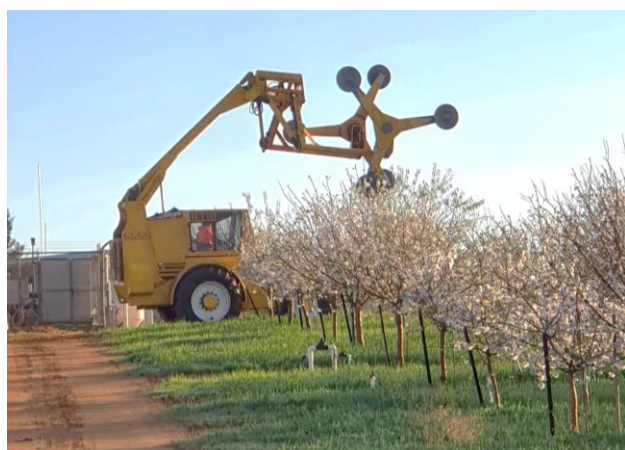
Figure 22 Dual boom hedger topper performing the hedging action at the start of the third leaf growing season.
