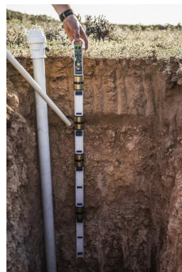
Figure 44 Image showing the EnviroSCAN probe sensors at different depths
