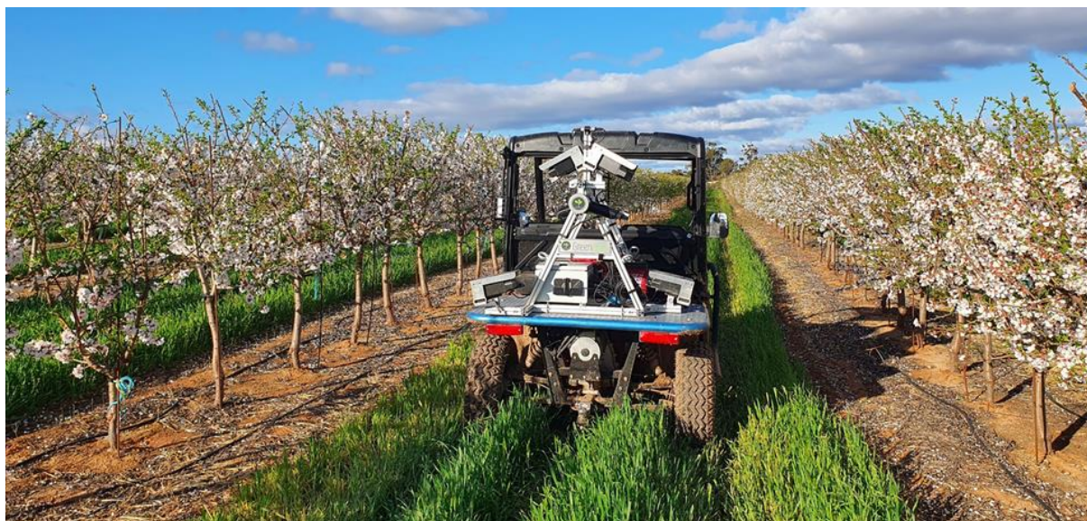
Figure 81 The Cartographer instrument mounted on an electric side-by-side vehicle and scanning the higher density plantings for development of the flower count prediction model
