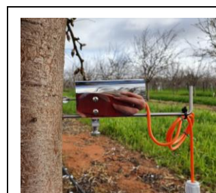
Figure 43 A trunk dendrometer installed on a tree in the higher density plantings
