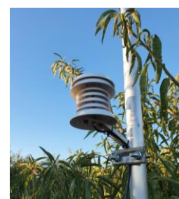
Figure 47 A TinyTag temperature probe installed at 2 m within a gill screen in the higher density plantings.
