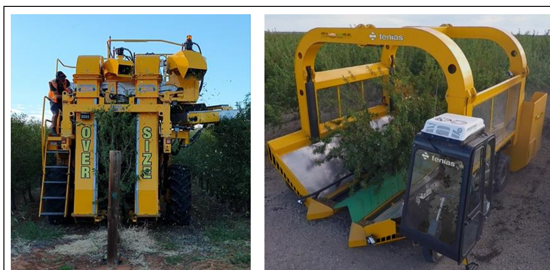
Figure 62 Mechanical over-the-row harvesters available for almonds
