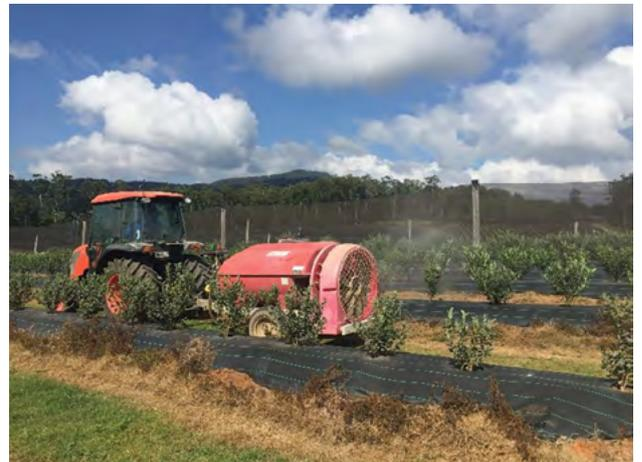
Figure 3. An axial air-blast sprayer. Photo: Melinda Simpson.
