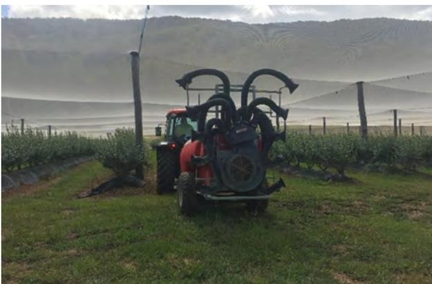
Figure 1. A ducted air sprayer. Photo: Melinda Simpson.
