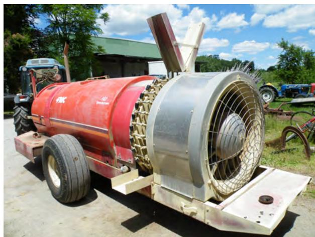
Figure 7. Deflectors on an air-blast sprayer. Photo: Sprayers 101.
