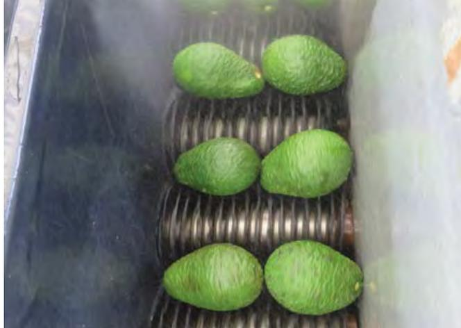
**Figure 7.** Hass fruit rolling over brushes under treatment sprays in the experimental-scale packingline. The equipment is ideal for treatment of whole tray (approximately 20 pieces) replicates of fruit, allowing for robust statistical analyses of data. Volumes of 80L can be used, and the tank and line is easily flushed between treatments so that multiple separate treatments can be applied in a few hours.
