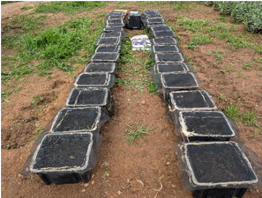
Figure 1: Field mesocosm used in Trial 2.
