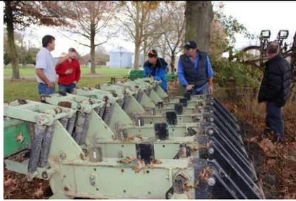
**Figure 22: Explaining the Orthmann strip till rig**
