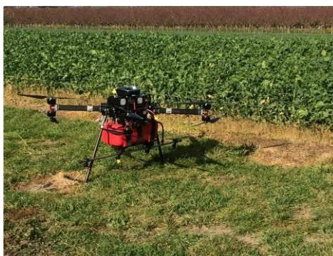
**Figure 12: UAV with 20l spray tank**
