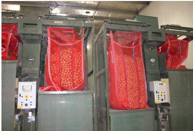
**Figure 20: One (1) tonne bags being filled for direct export.**
