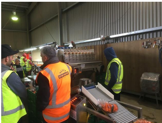
Automated carrot bagging machine that uses sensors to select groups to drop carrots into the bag to get the closest desired weight.
