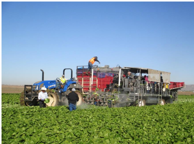
Automated Harvesting's machinery that uses high-pressure water jets to automatically harvest cos lettuce.
