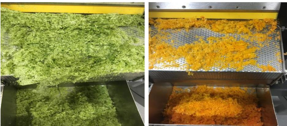
**Figure 17. Drum dried broccoli (left) and carrot (right) powders**
