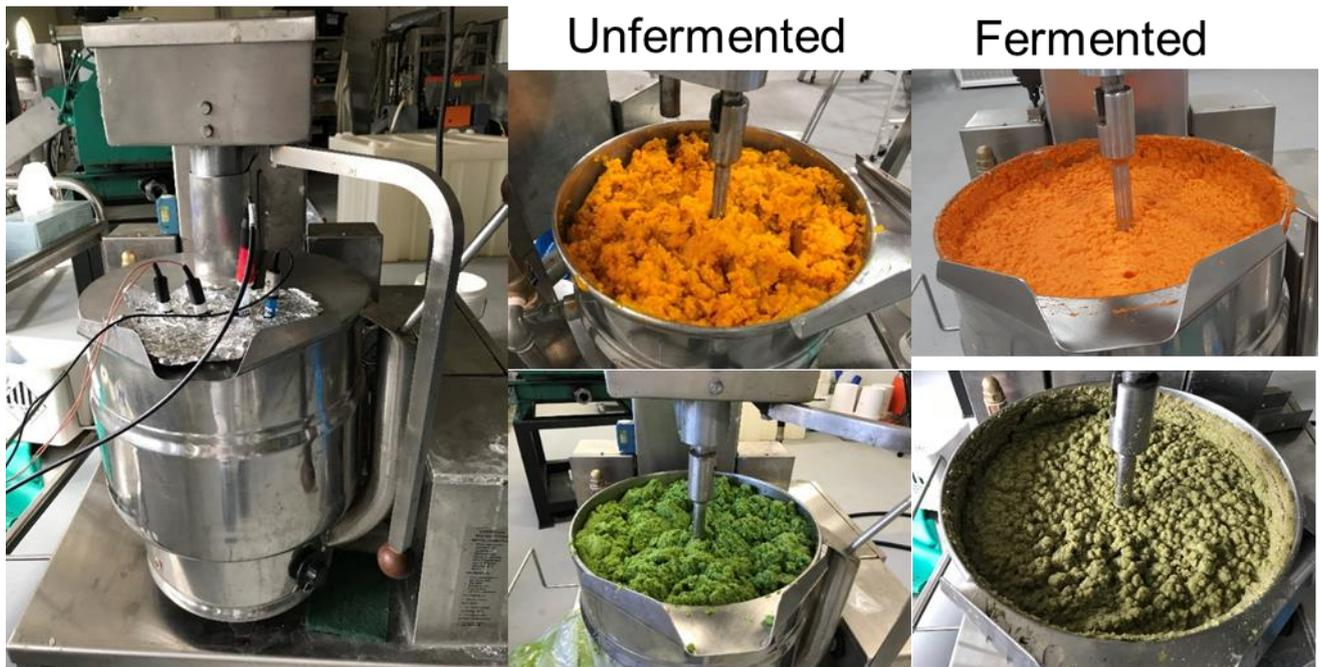
Figure 32 Experimental set up for small pilot scale fermentation trials of carrot and broccoli puree showing the Groen kettle used as fermentation tank and samples at the beginning and end of fermentation.
