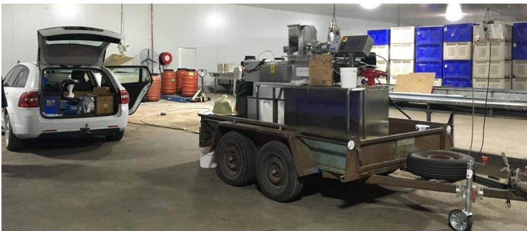
**Figure 25** Extruder is set up on arrival at the site and connected to power and water supply.
