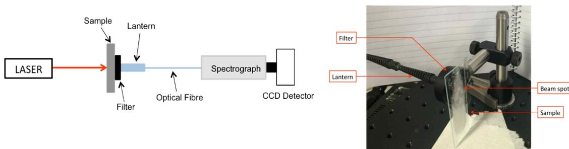
Figure 2 - Raman set-up arrangement (left), illuminated sample and light collection with the lantern (right)
