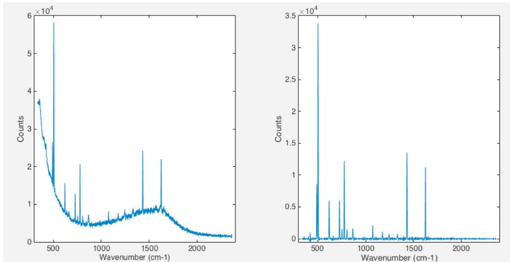
Figure 1 - (Left) Raw Raman signal from Paracetamol. (Right) Signal after post-processing.
