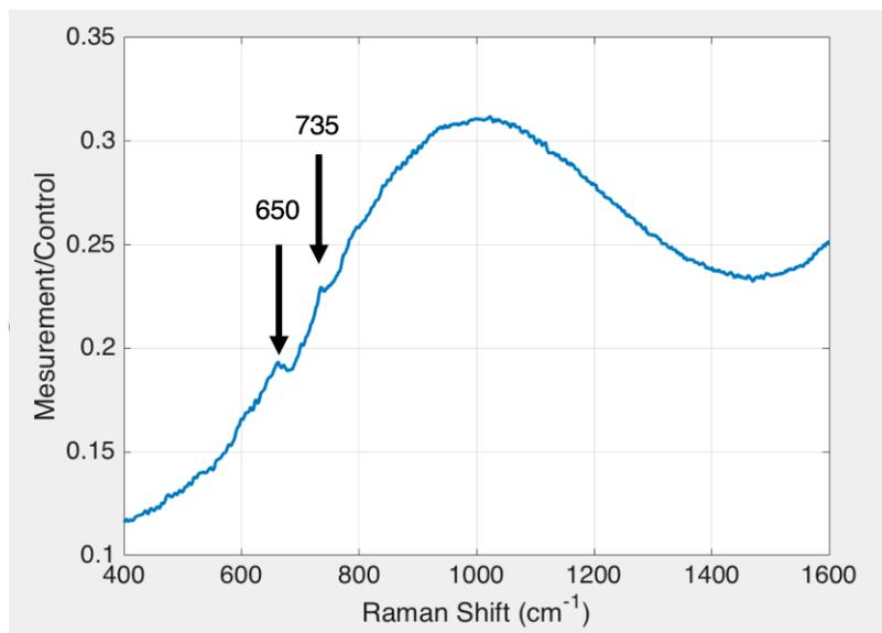
*Figure 6 - Differential measurement of Raman spectra obtained of Salmonella contaminated spinach. The two labelled peaks are considered indicative of bacteria presence.*
