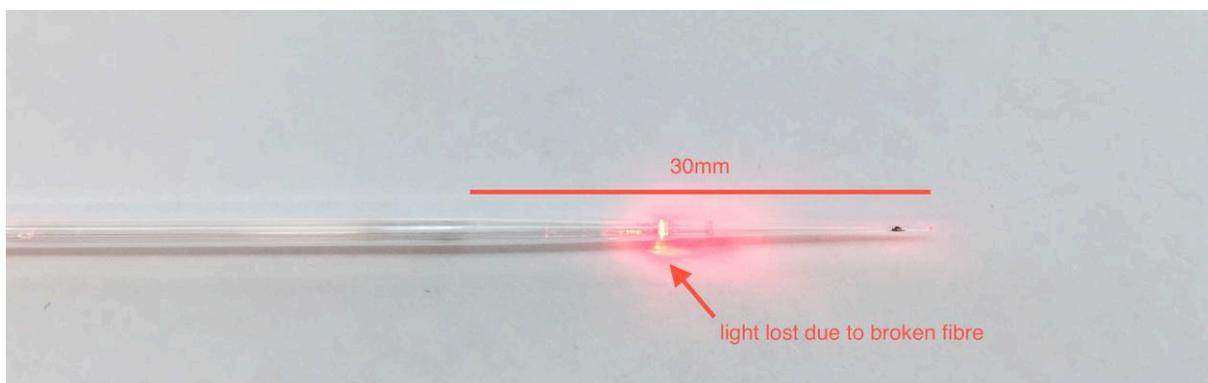
Figure 2 - Image of an unsuccessful fibre bundle. The multimode delivery fibre broke mid transition. As result all the light from the excitation laser is lost.
