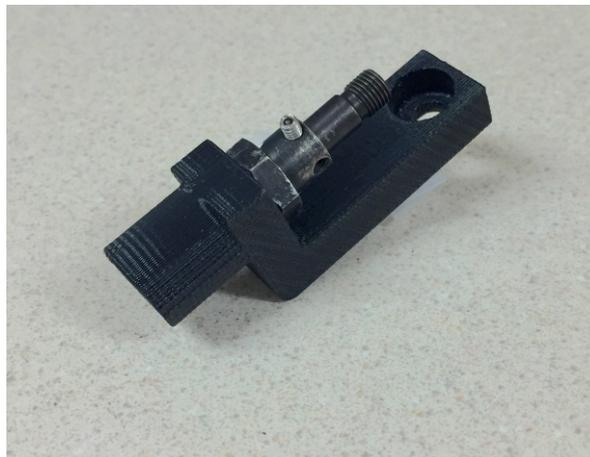
*Figure 4 - Raman Probe holder, includes baffle to indicate focus position and block stray light.*
