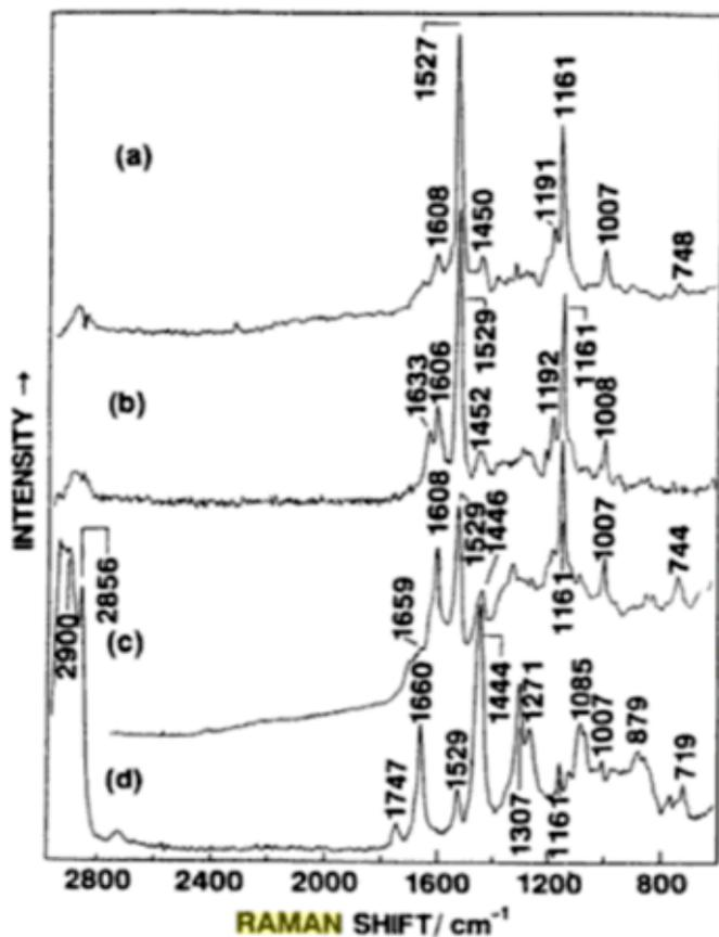
**FIGURE 20** FT-Raman spectra of (a) fresh spinach leaf, (b) peel of mandarin orange, (c) new leaf Japanese tea, and (d) hen's yolk. (Reproduced from Ref. 25 with permission. Copyright © 1992, Society for Applied Spectroscopy.)
