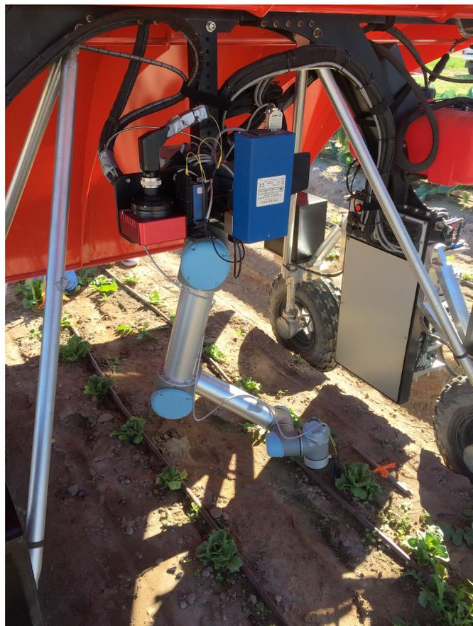
Figure 11 – ACFR's Ladybird Robot fitted with the Raman sensor probe. The laser, CCD and electronics have been integrated with the Ladybird's frame and electrical power distribution.
