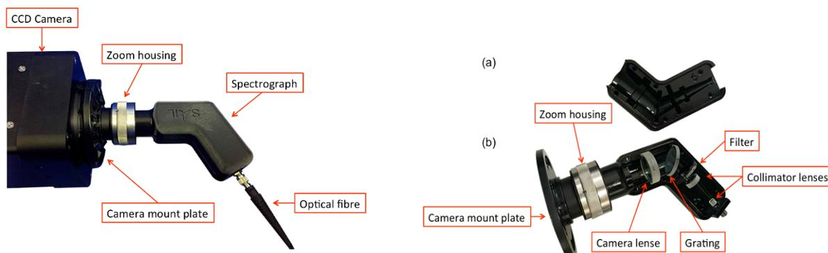
Figure 1 - Raman spectrograph mounted on CCD camera. (Left) Assembled. (Right) Disassembled.
