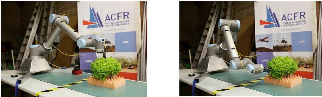
*Figure 7 - Raman sensor mounted to the robotic arm and demonstration movement between two sample points.*
