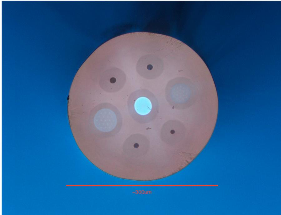
*Figure 3 - Our combined Raman delivery/collection bundle. The central feature is the multimode delivery fibre that was coupled to the Raman excitation laser. To either side are the photonic lanterns formed from a multicore fibre (the SM cores are just visible).*
