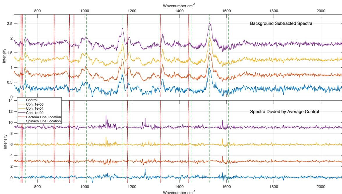
Figure 10 - Top Panel shows the sample background subtracted spectra of the inoculated spinach leaves and the control. Bottom Panel shows each spectrum divided by the average of all control spectra. A difference from the bacteria line would be considered evidence of detection. Shown in both are vertical lines that indicate the position of spectral lines associated with Bacteria (red) and spinach (green).
