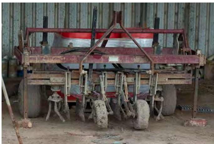
Figure 3 A 'Weedfix' inter-row cultivator, used on the farm in less mature leek crops for shallow cultivation within the crop bed.
