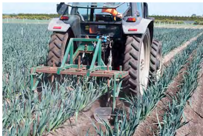
Figure 4 A customised inter-row cultivator, set up to the specific bed and row spacing used on the farm. The cultivator is being used within a more mature leek crop to cultivate within the crop bed as well as the wheel tracks.
