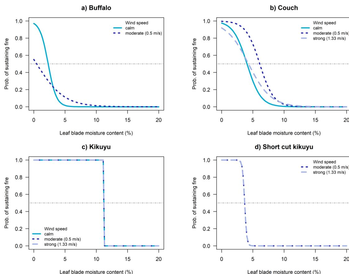
**Figure 12** Univariate logistic regression plots for point ignition sustained combustion in buffalo, couch, kikuyu and short cut kikuyu turf based on leaf blade moisture content in different wind conditions.
