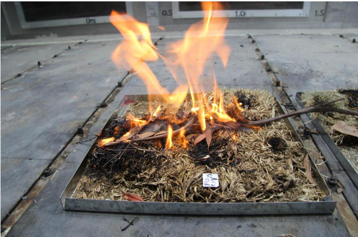
Figure 14 Litter burning on top of a sample of buffalo turf that did not sustain point ignitions (leaf blade moisture content 5.5% ODW)
