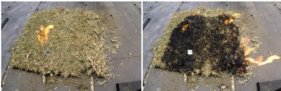
**Figure 8** Sustaining ignition in buffalo grass turf with a strong wind speed (ignition number 167). Unburnt fuel is visible underneath the burnt tips (right)
