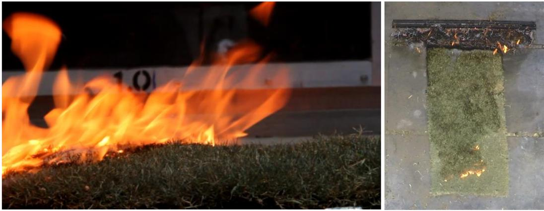
Figure 18 Example of spreading fire burning across the tops of the turf layer. Spread sustainability test 18 (Table 5) burning in couch, as viewed from the side (left) and above (right).
