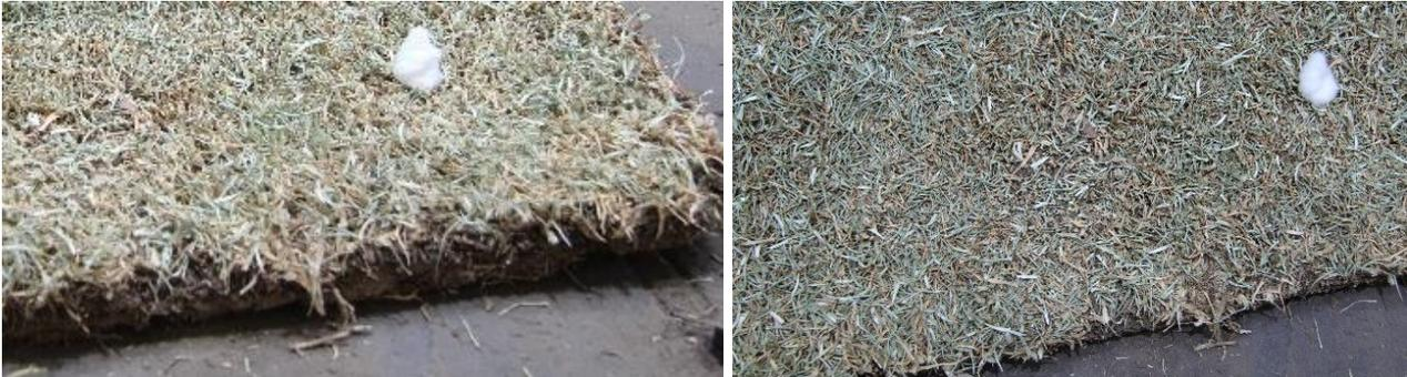
Figure 3 Example of short cut kikuyu turf. The mean blade height of this sample was 10.3 mm.
