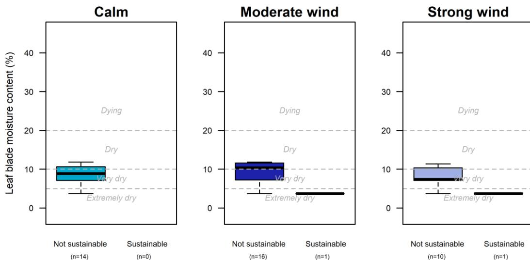
**Figure 11** Boxplots comparing the leaf blade moisture content during non-sustaining and sustaining point ignition tests in short cut kikuyu turf under the different wind conditions. Black lines show the plot median, coloured boxes show the range between the upper and lower quartiles. Whiskers show the range other than outliers (circles) that are more than 1.5 times the upper quartile, or less than 1.5 times the lower quartile.
