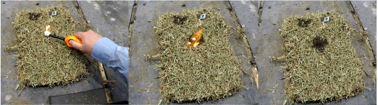
*Figure 2 Point ignition experiment sequence*
