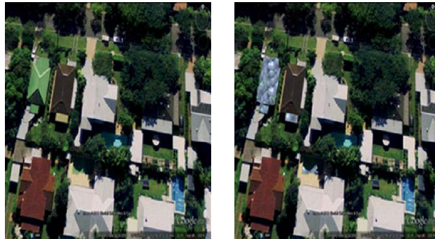
Figure 2. (a) Left - Original Image (Eye Alt 100m) showing green roof (top left corner) which presented a potential form of error in estimating the percentage turf cover and; (b) Right - after processing in Adobe Photoshop.
