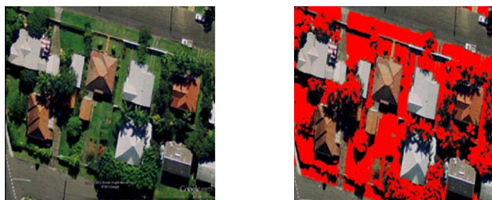
Figure 1. (a) Left - Original Image (Eye Alt 100m) and (b) Right - after analysing in Sigmascan Pro software for turf cover.
