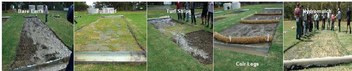
Figure 3: Scenarios (from left to right), bare earth, full turf, turf strips, coir logs and hydromulch
