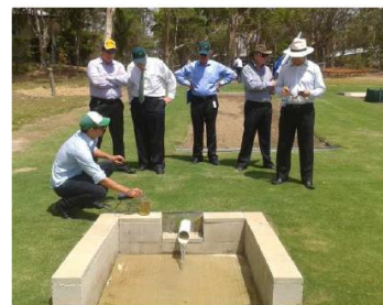
Figure 3. (Top) Demonstrating sediment capture capabilities of turf (Bottom) measuring turbidity
