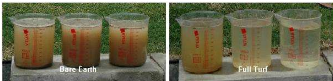
Figure 4: Collected runoff at the three intervals for the bare earth and full turf scenarios
