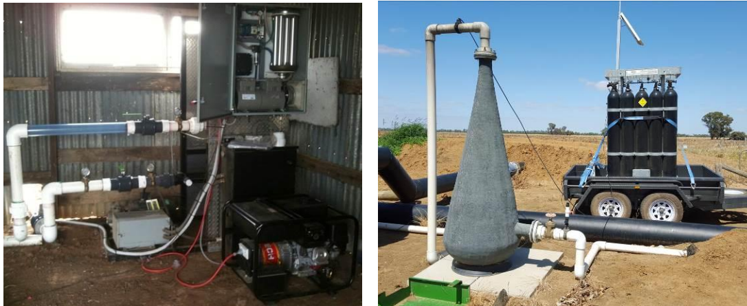
Figure 1. Pressure swing adsorption system (left) and direct compressed gas injection system (right) used to generate high dissolved oxygen concentration in irrigation water.
