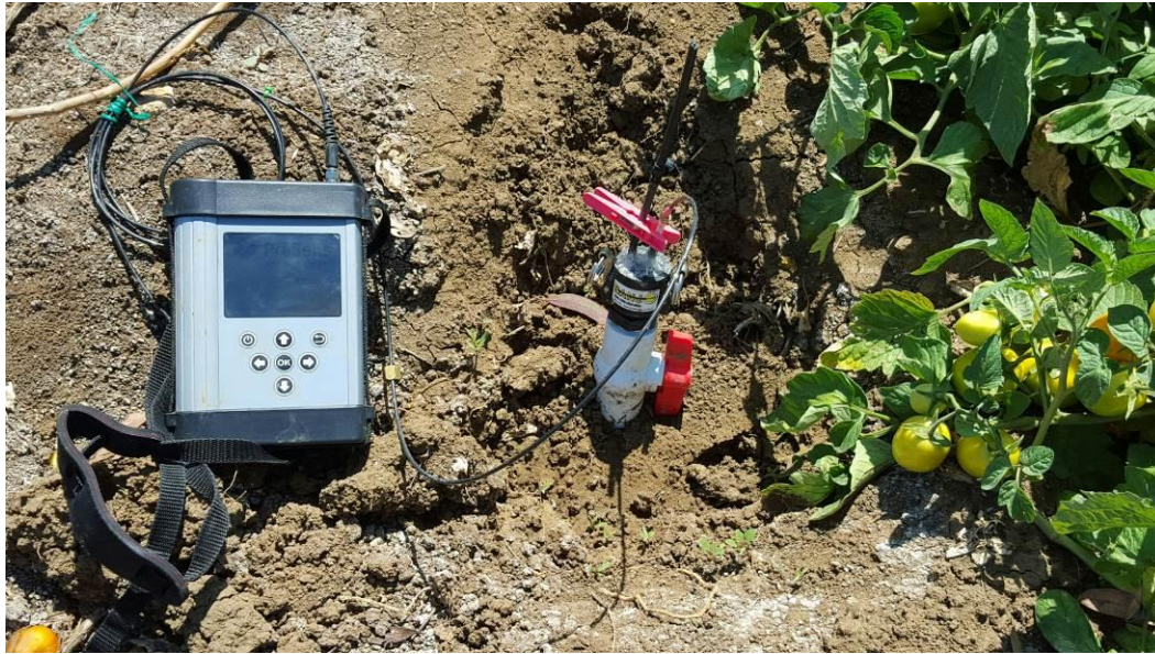
Figure 2. Sampling port assembly with fibox-3 oxygen meter connected.
