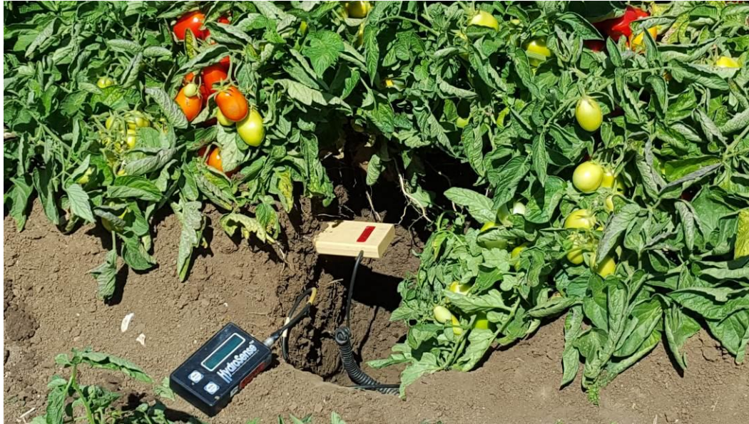
Figure 3. Hydrosense soil moisture monitoring probe inserted in soil profile.
