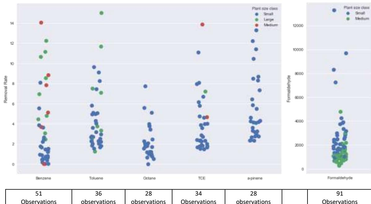
Figure 4: relationship between contaminant removal rate and plant size
