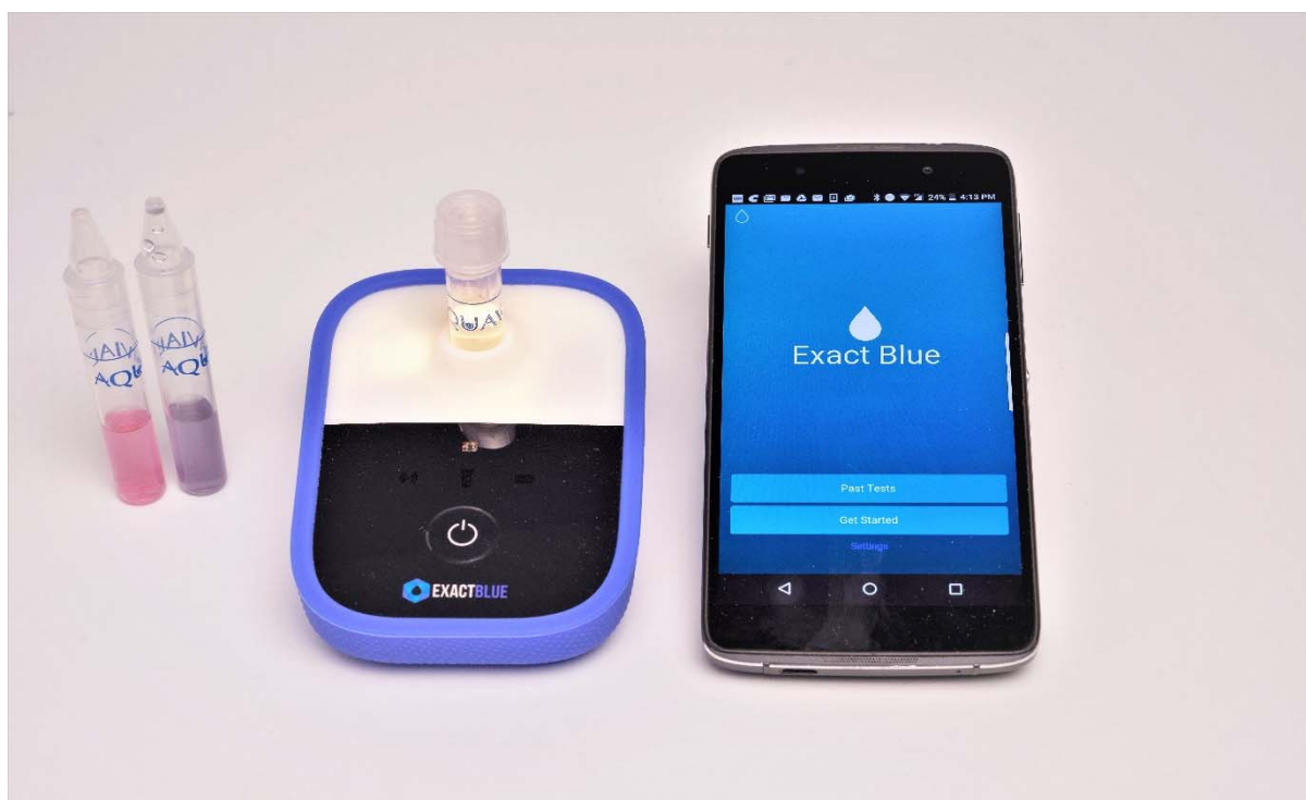
Figure 3. Detection of bacterial contamination in water samples using the Genemis AquaVial test kit and the Exactblue device.
