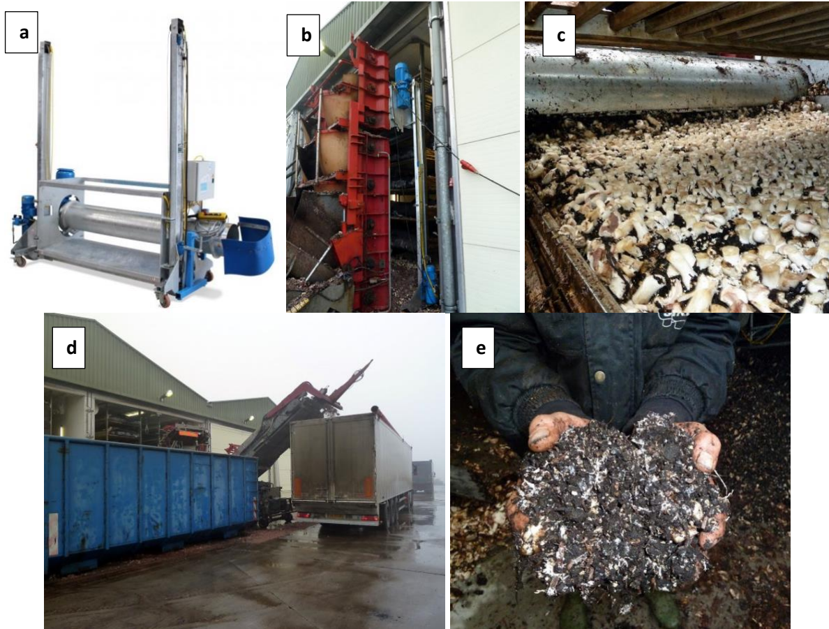
Figure 52. The Mush Comb unit (a) is used to separate the casing from compost during room unloading. The separator is used with a multi-arm emptying machine (b) as the crop is removed after final harvest (c). Conveyors take compost into the waiting trailer, while casing is diverted to a container at one side (d). The separated casing soil (e) and compost can then be recycled or used for other purposes. Photos by Mush Comb ( www.mushcomb.com ) and The Mushroom People ( www.themushroompeople.com ).
