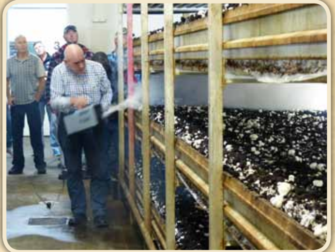
Trainers Tip(from Jan Gielen): When you want to see the detail you put the smoke across the bed. You look at the direction of the air and the velocity of the air and you do this on all levels. Editors Note :This machine was a fog machine purchased from Dick Smiths.
