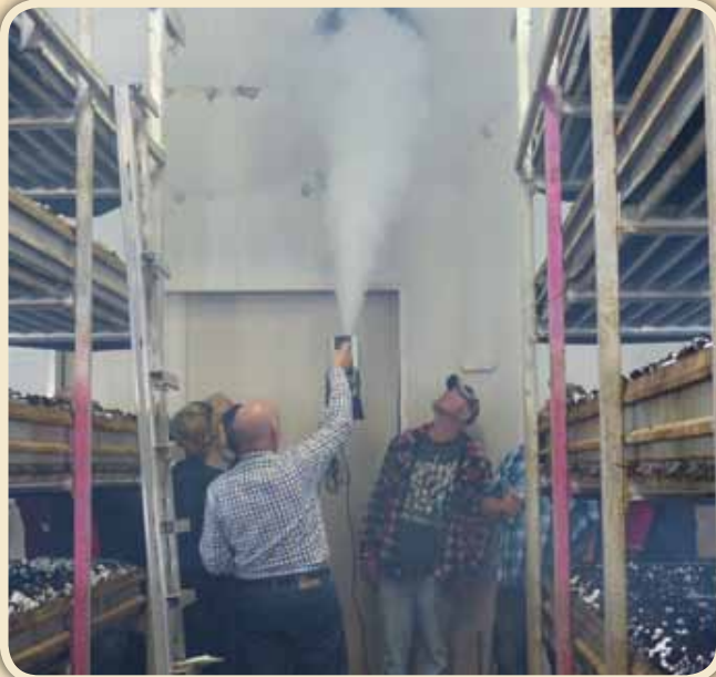
Trainers Tip (from Jan Gielen): Directing smoke into the return duct can give you a quick scan of the air distribution.
