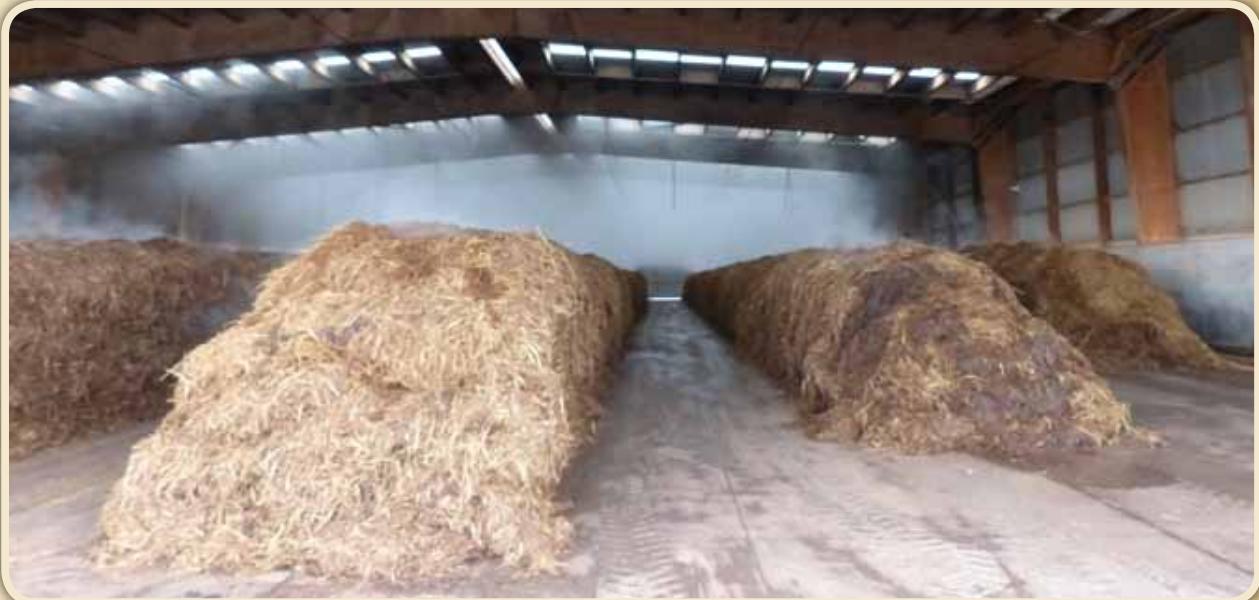
"We call the next stage in the shed our prewet. The 4 ricks have air lines under them and we turn twice for blending."
