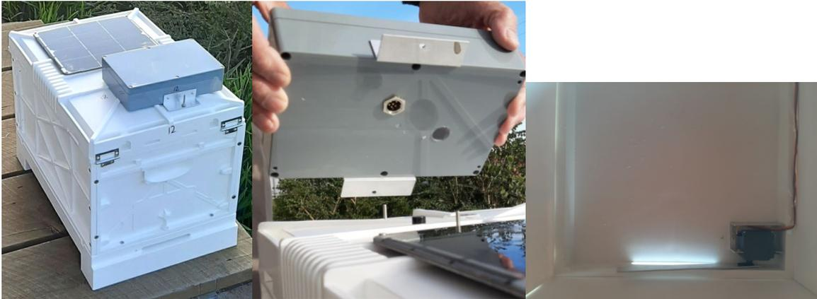
**Figure 12** Design of the RCB-V2 (2020 design). The box is the industry preferred Nuplas catchbox, the solar panel is half the size of the original, the electronics are in a detachable weatherproof box, and the internals of the catchbox have been simplified, with minimal (as possible) wiring.
