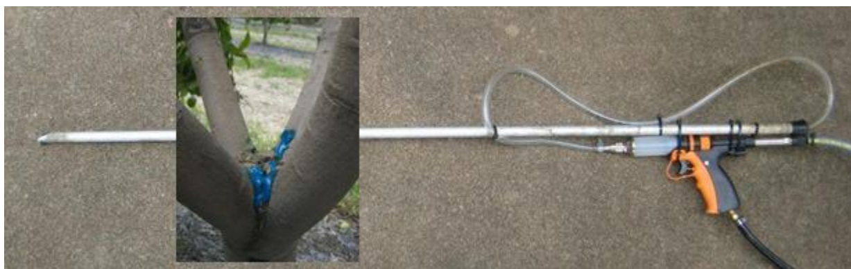
Figure 7. Hand lance for applying fruit fly bait to mango trunks (figure insert describes a measured amount of bait gel applied to crotch of the tree).
