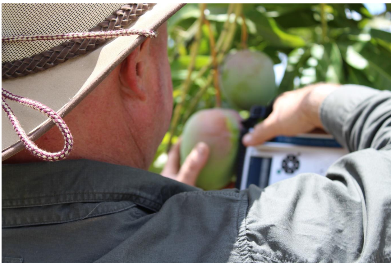
F. NIR produce quality meters being used by a grower to measure %DM of harvested fruit 30 November 2017 in the Mareeba region, Queensland.
