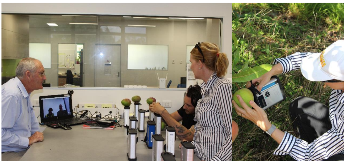
E. NIR produce quality meters being calibrated using a selection of KP, R2E2, Calypso and Honey Gold fruit with a range of maturities 17 November 2017 at UCQ Rockhampton, QLD. Selecting fruit for calibration on the day.
