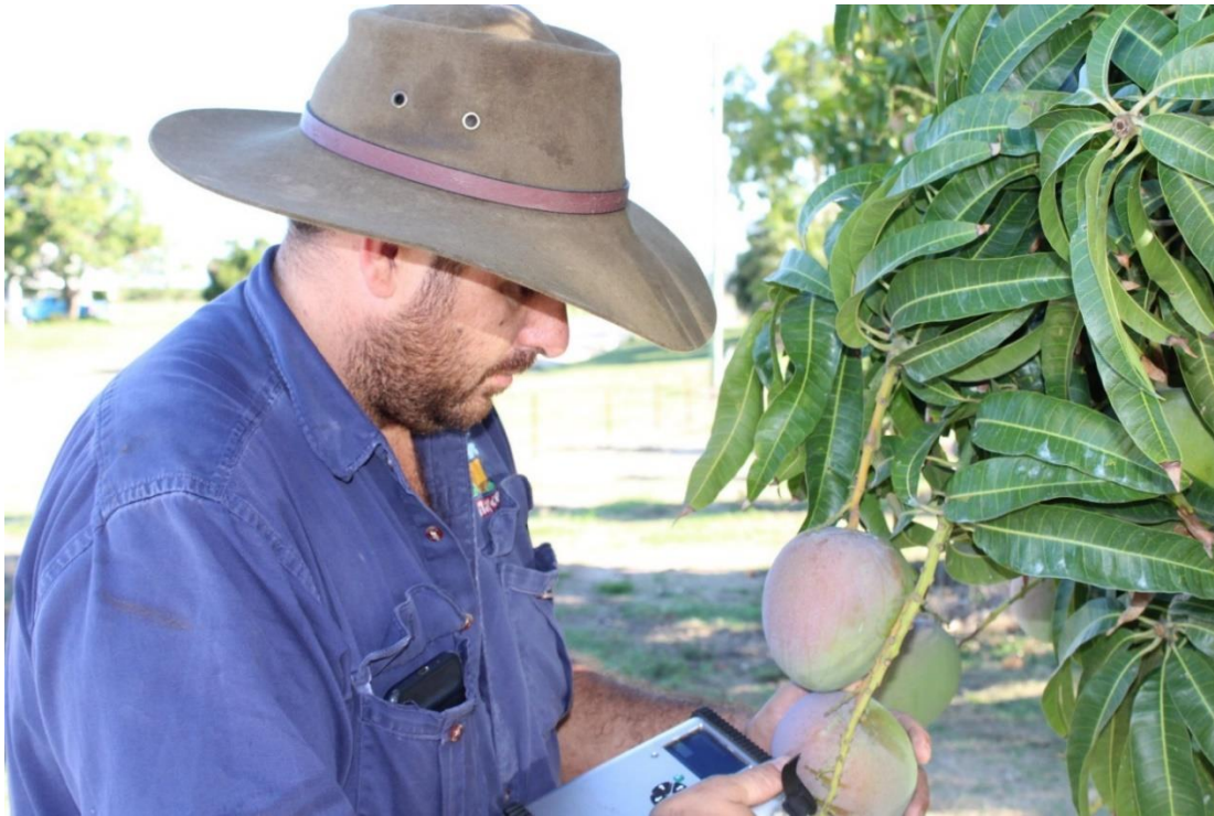
C. NIR produce quality meters being used by grower Ben Martin to measure %DM of fruit still developing on the trees 26 October 2017 in the Bowen region.
