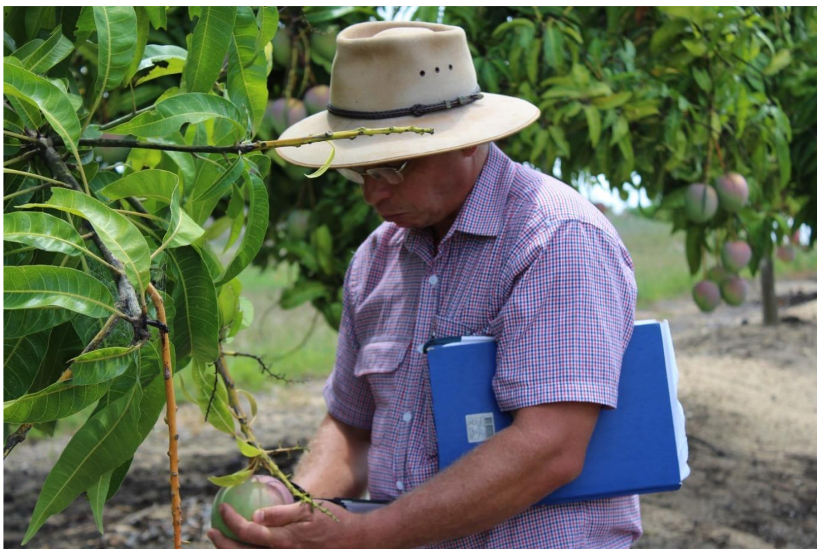
G. NIR produce quality meters being used by a grower's consultant to measure %DM of harvested fruit 30 November 2017 in the Mareeba region, Queensland.
