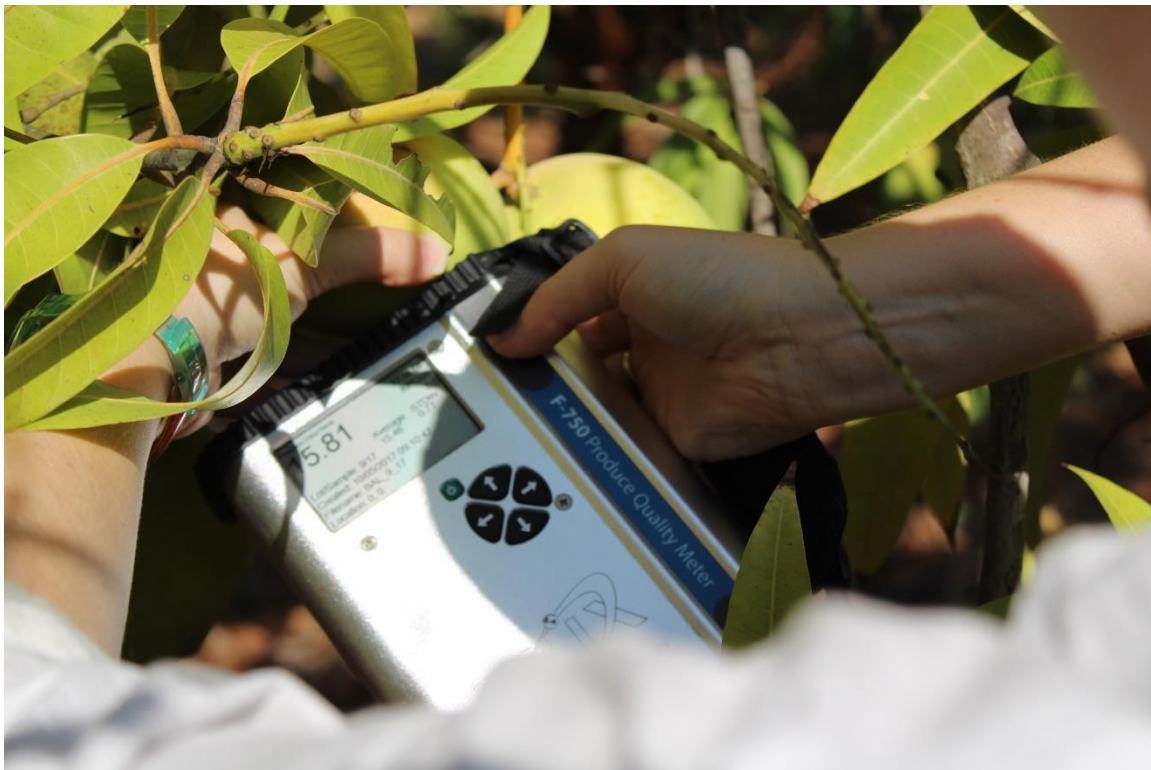
B. NIR produce quality meters being used by project staff to measure %DM of harvested fruit during 5 October 2017 in the Katherine region, NT.
