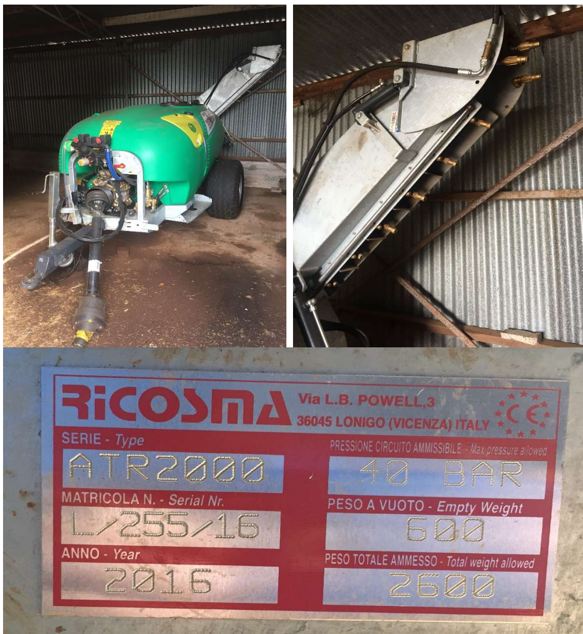
Figure 2.5.2.7.: NSW DPI 2000L trailer mounted Tuffass® spray unit details, and canon nozzle structure, and manufacturing plate.
