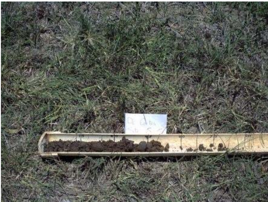
Fig 6. Site 5. Grey, sandy, clay loam to 45cm over yellow red clay with ferruginous nodules present. In contrast to the other sites, the clay at depth in this site was wet and very sticky from 45cm.
