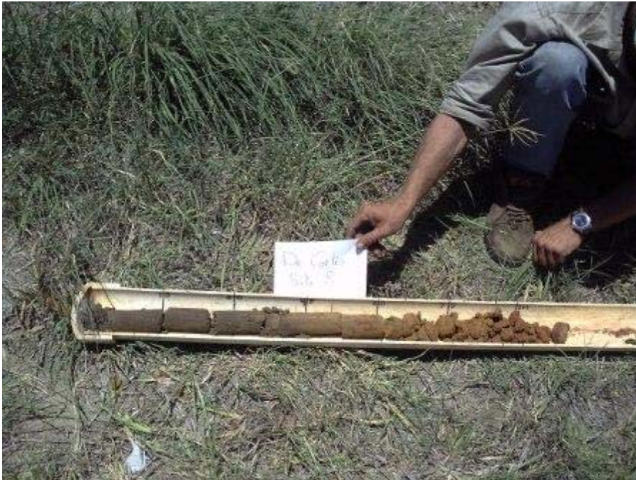
Fig 9. Site 8. Grey, sandy, clay loam to 40cm over yellow, light clay to 60cm, becoming medium yellow/red clay from 75cm to 1m.
