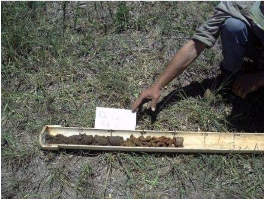
Fig 7. Site 6. Grey, sandy, clay loam to 35cm over yellow, light becoming medium clay. Conspicuous ferruginous band at 50cm becoming medium red clay with ferruginous nodules present.
