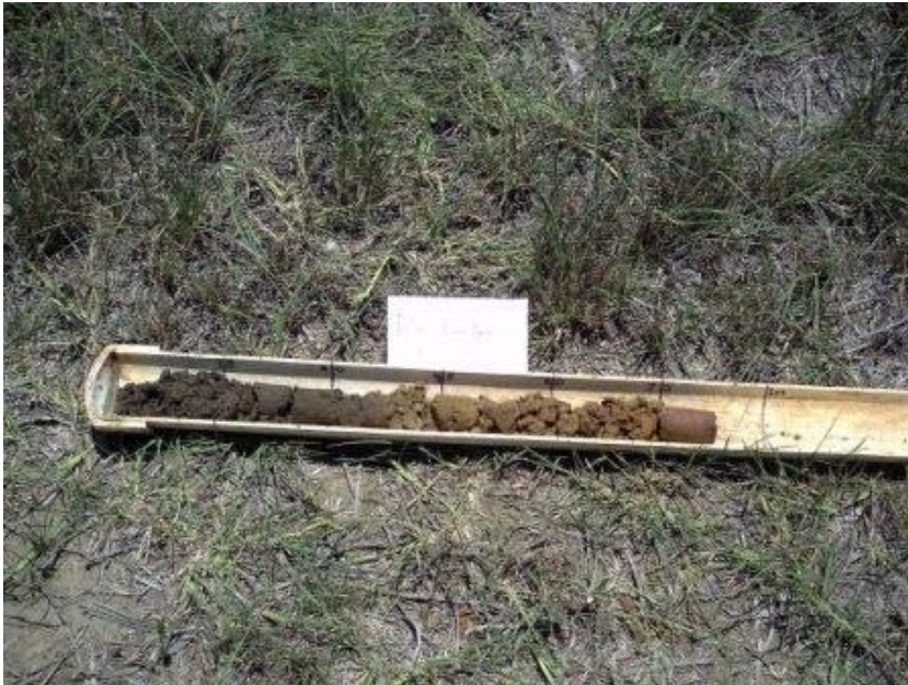
Fig 3. Site 2. Grey, sandy, clay loam to 30cm, over light becoming medium yellow clay B horizon with significant ferruginous band present at 50cm. Heavy, red/yellow clay from 75cm which was very dry and which the machine could not penetrate.
