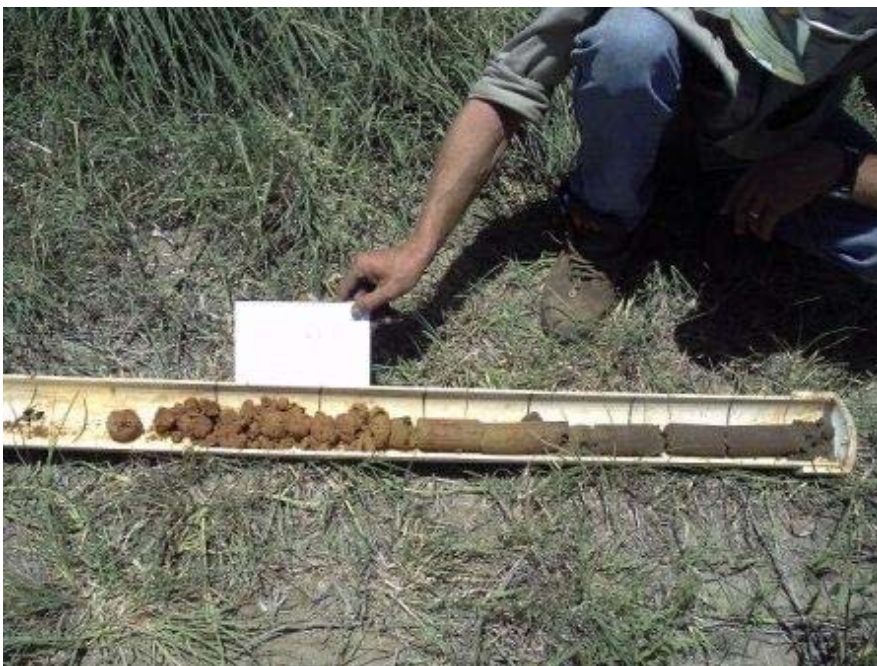
Fig 8. Site 7. Grey, sandy, clay loam to 35cm over yellow, light to 50cm, becoming medium yellow/red clay from 50-80cm. Medium red clay from 80cm containing ferruginous nodules.
