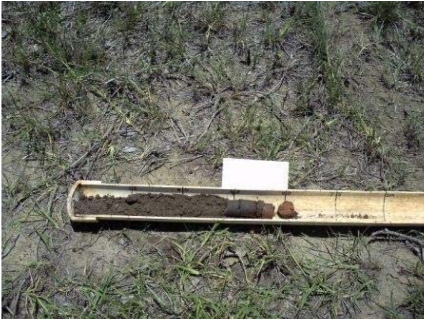
Fig 5. Site 4. Grey, sandy, clay loam to 40cm, light brown clay to 45cm Strong ferruginous band present at 50cm with heavy red clay. Very dry could not penetrate red clay.
