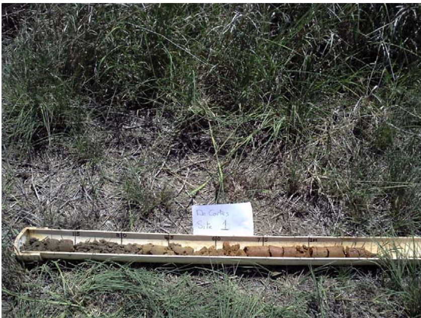
Fig 2. Site 1. Grey, sandy, clay loam to 50cm over light red clay becoming medium clay to B horizon to 1.2m, Ferruginous nodules present from 1m
