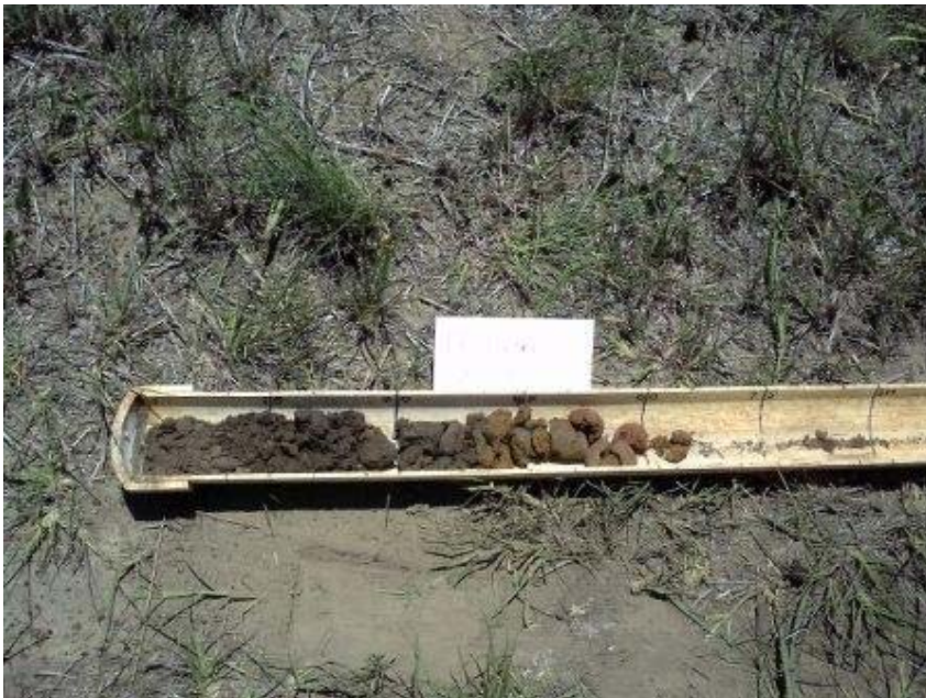
Fig 4. Site 3. Grey, sandy, clay loam to 35cm, over medium yellow clay B horizon. Strong ferruginous band present at 50-60cm with heavy red clay. Could not penetrate past 60cm..
