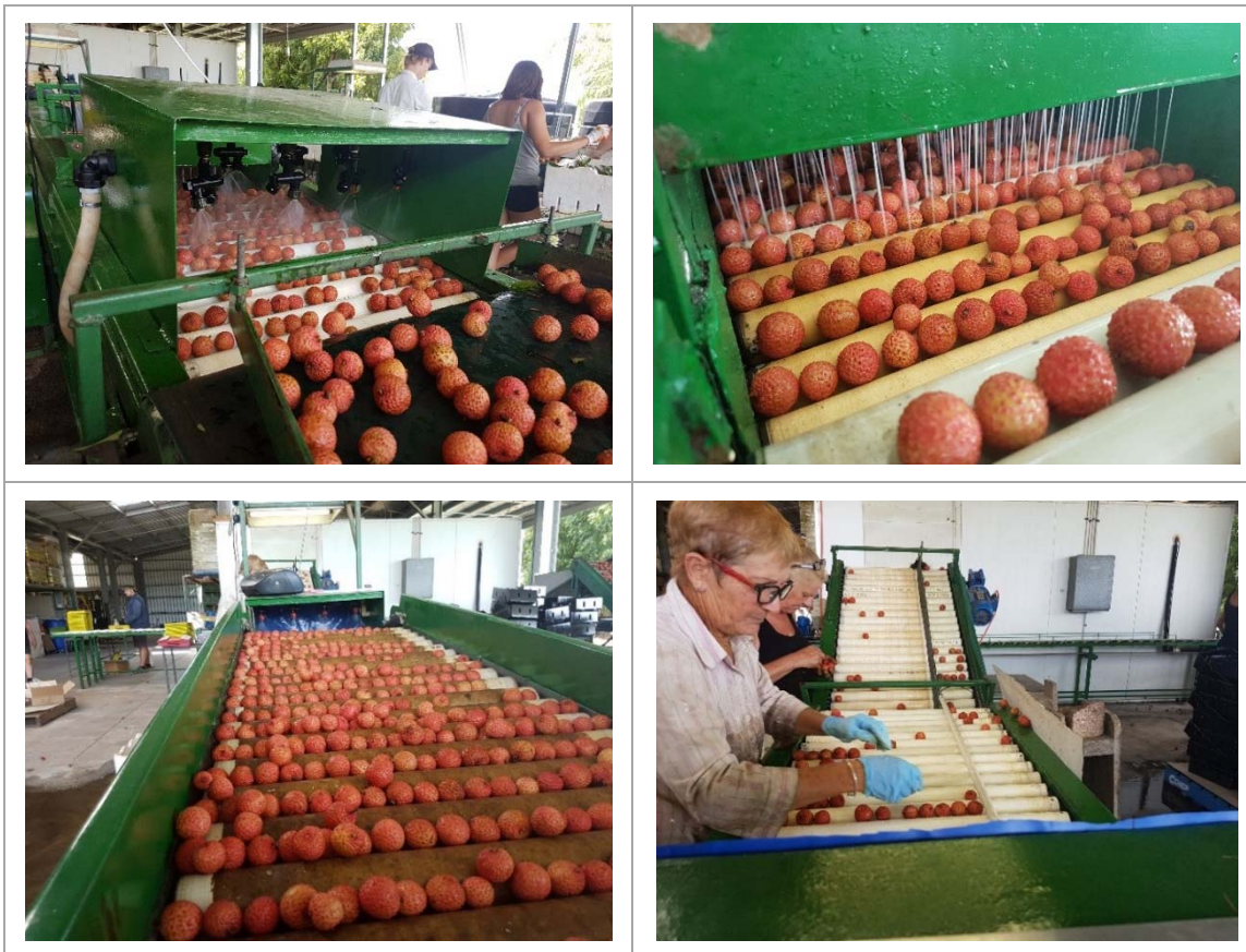
Plate 19. Components of the commercial oil/spray prototype ( from left to right ): Top row - pre-wash; oil flood spray; Bottom row - Oil drip line (two minute transit) until post oil application spray at the far end of the conveyor; final sorting prior to packaging.
