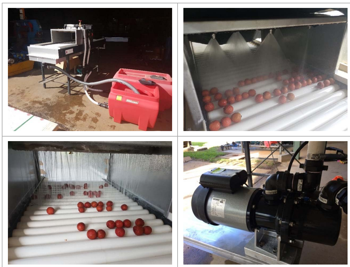
Plate 17. Experimental prototype oil flood spray and high pressure water washing (from left to right): Top row - Roller conveyor with spray hood, water and oil tanks; Twin fan nozzle water spray for pre or post oil application (5 fan nozzles, 1.11 L/s at 13 psi); Bottom row - Flood spray for oil application (0.63 L/s at 0 psi); Mono helical rotor pump used for oil application.
