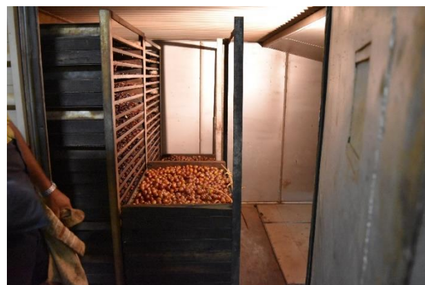
Photo 8: Ultrasonic treated fruit prior to drying in a commercial dehydrator. Photo 9: The placement of the fruit in the drying tunnels.
