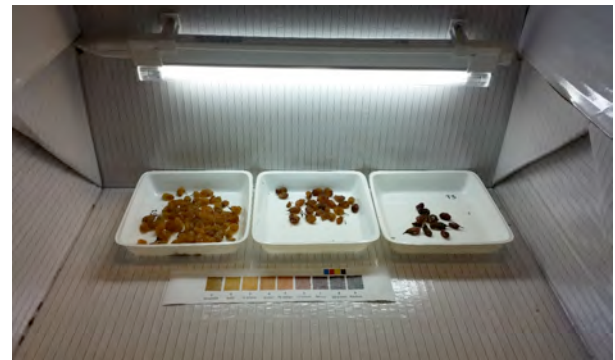
Fig. 1. Light box setup for assessing color of raisins
