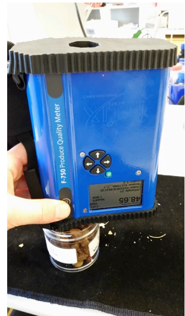
Figure 6. Using the Felix F-750 to analyse grape samples
