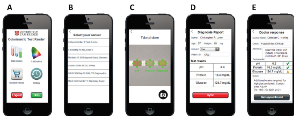
Figure 20 - Screenshots of the IOS app developed by Cambridge university. A-Main menu, B-Sensor types, C-Image of the test strip, D-Diagnostic test results, E-User instructions (Yetisen et al. 2014).
