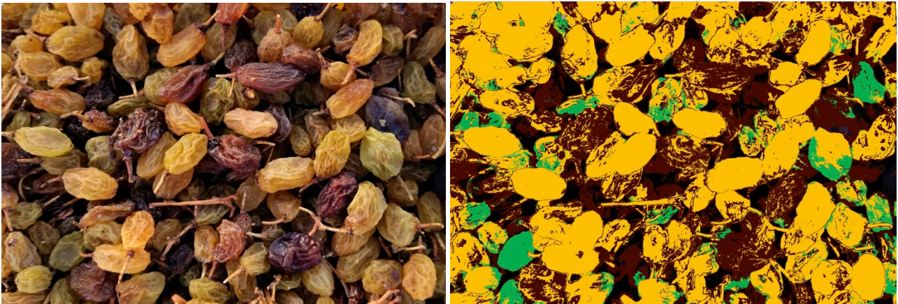
Figure 24 - ImagePro analysis showing original (left) and divided into brown, green and yellow fruit (right). The software can provide an analysis of the percentage of each object within the image.
