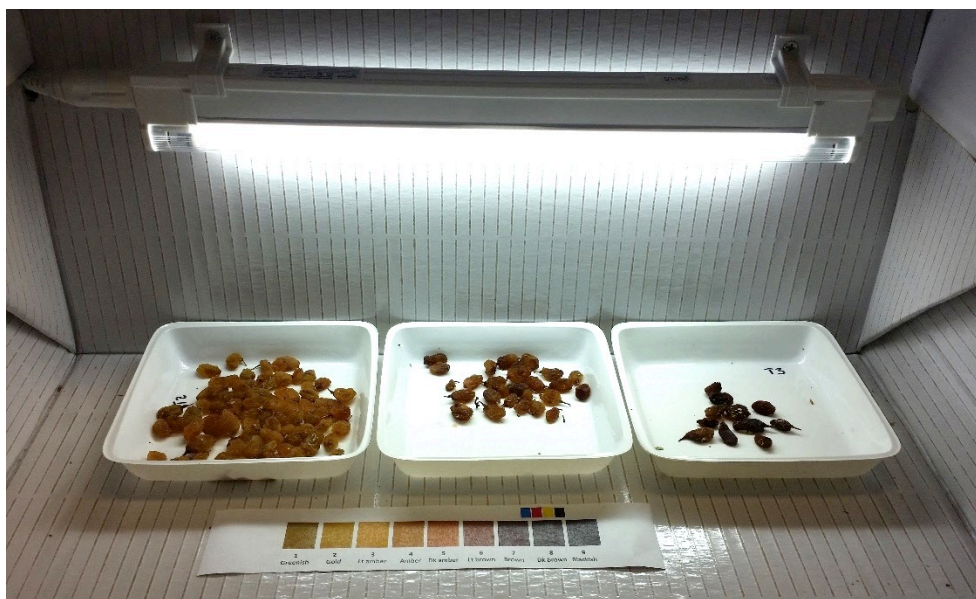
Figure 5. Light box setup for assessing colour of sultana colour
