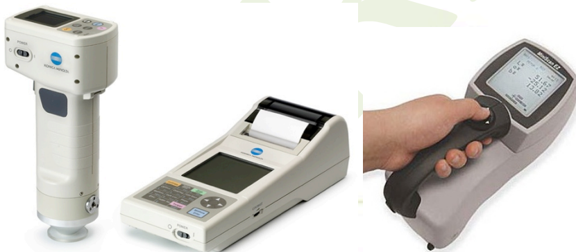
Figure 7 - Konica Minolta CR-400 chroma meter and the HunterLab MiniScan EZ.
