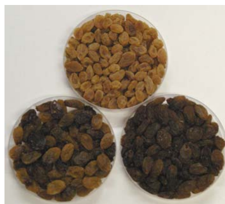
Figure 1 DVF samples used to calibrate the Minolta Chroma Meter and the ColourVision systems
