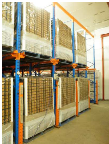
Figure 37. Pallet covers over pallets of blueberries in storage. The specially designed plastic cover will generate the optimum atmosphere within the cover for long term cold storage.
