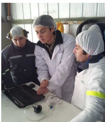
Figure 17. Demonstration of the artificial electronic cherry by Ignacio Rojas from AgVision S.A. for recording impacts in the cherry packingline.
