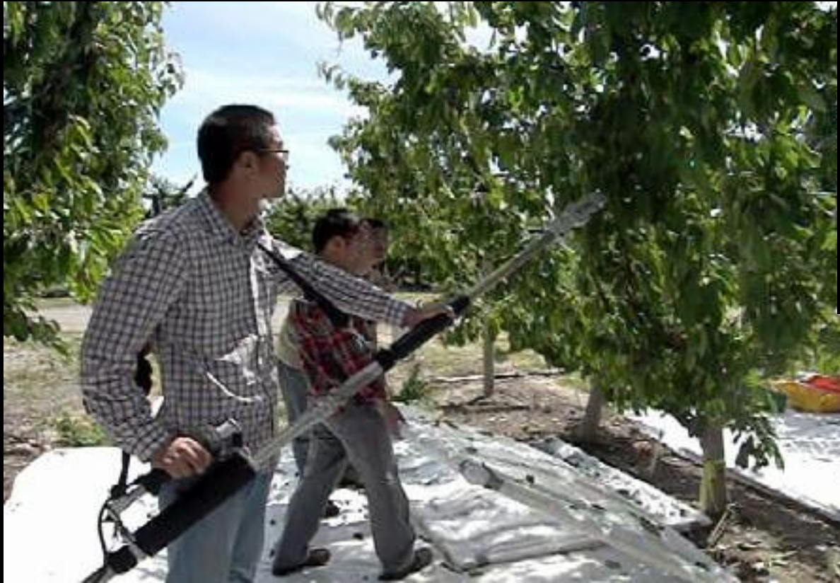
Shake-and-catch harvest testing
