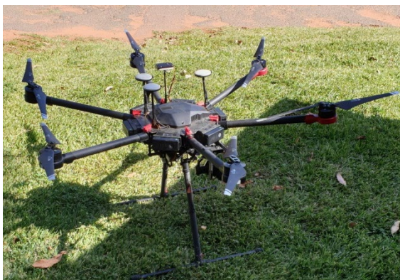
Figure 6.4: Drone used with multi-spectral camera operated by StevTech in 2020. Photo: Dr Tahir Khurshid.
