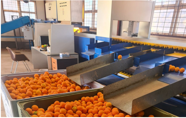
Figure 2.4: Fruit were weighed, counted and graded into different size classes for each tree with a commercial Colour Vision grading machine at Dareton. Photo: Dr Tahir Khurshid.
