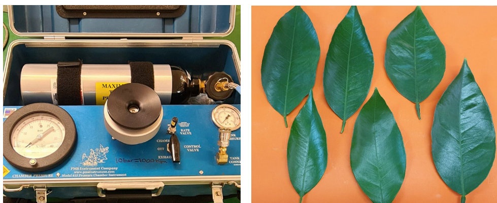
Figure 2.2: Pre-dawn stem water potential was recorded in a pressure chamber on fully expanded leaves. Photo: Dr Tahir Khurshid.
