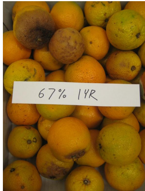
Figure 22: Mould development on overstored fruit (67%1year - 2011)
