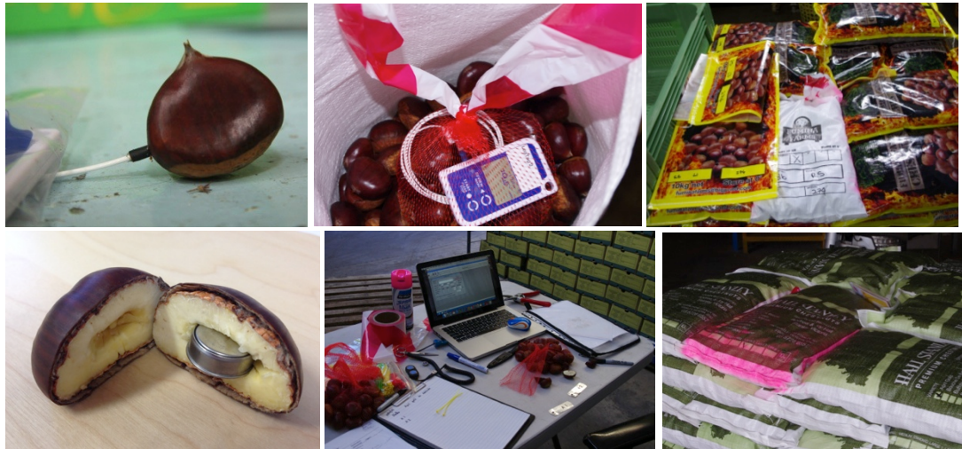
Figure 2 - Setup of temperature data loggers for chestnut supply chains using LogTags with probes (top) or i-buttons (bottom)
