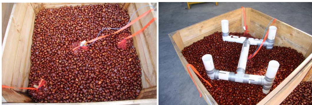
Figure 5 - Installation of weighed bags of chestnuts and loggers in a standard wooden bin (L) and wooden bin with ventilation pipes.
