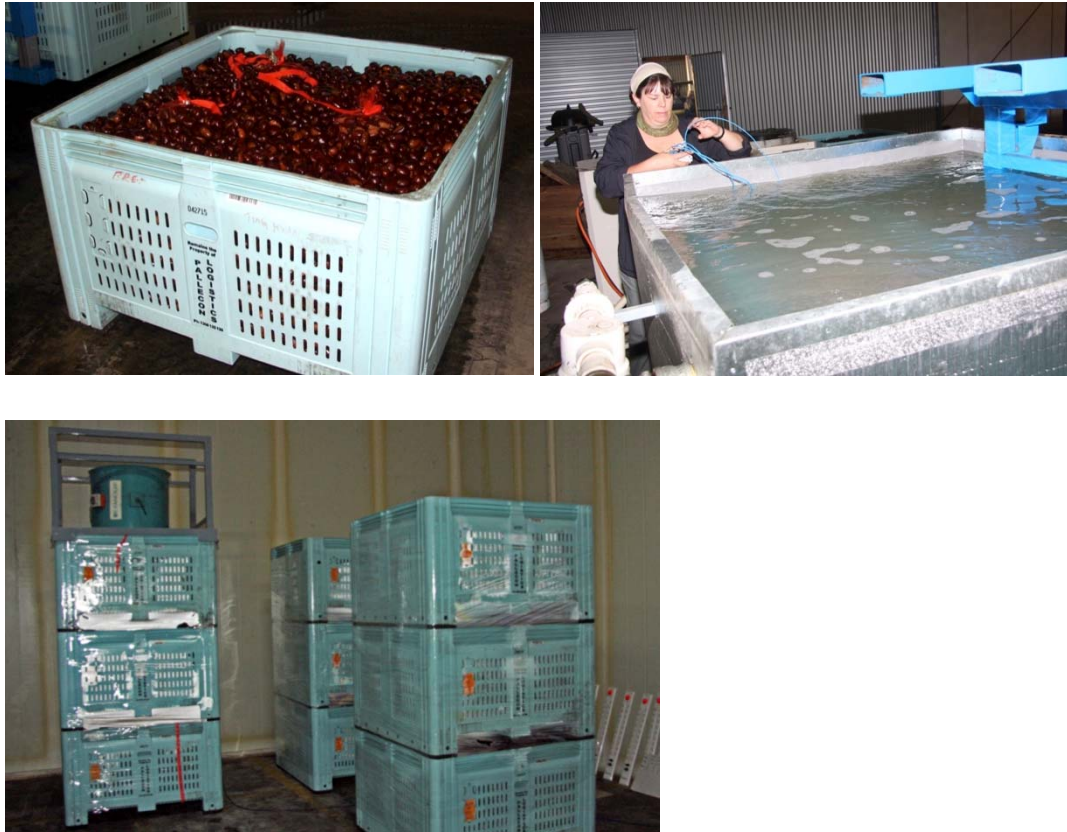
Figure 8 - Cooling systems used by Grower 3 included; room cooling in plastic bin, hydrocooling, and a forced air system
