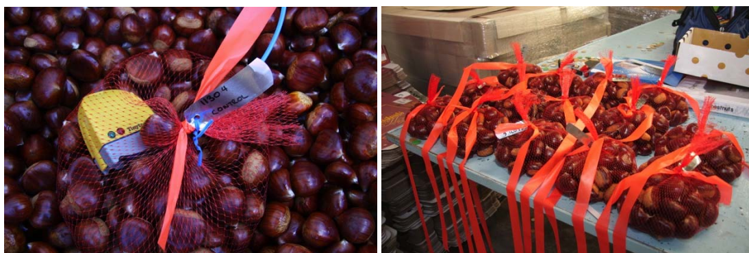
Figure 1 - Temperature dataloggers used to measure cooling rates. These included Logtags (top row), Hobo data loggers (centre row) and Tinytags (bottom left). Chestnuts with probes inserted were placed in mesh bags containing approximately 1kg of fruit, secured and marked with flagging tape (bottom right)
