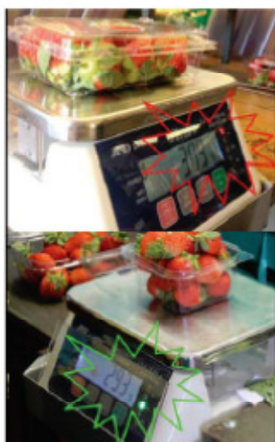
Figure 3. Examples of Pass and Fail scale outputs (limits set between 288g to 308g).
