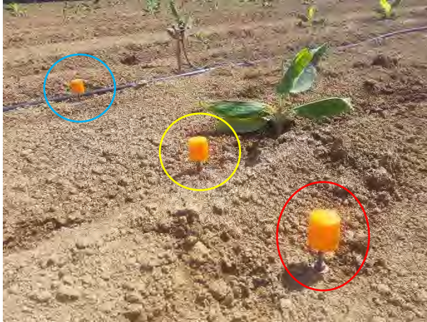
Figure 23: Three erosion pegs were installed on the southern side of each ground cover treatment and replicate. One peg near the irrigation line (highlighted blue), one in the middle of the southern side (yellow) and another peg installed on the outside shoulder of the bed (highlighted in red)
