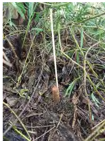
Figure 42: Image capture of erosion pegs following completion of the plant crop harvest. The level of deposition was recorded by measuring the distance between the washer and soil surface (using a skewer)
