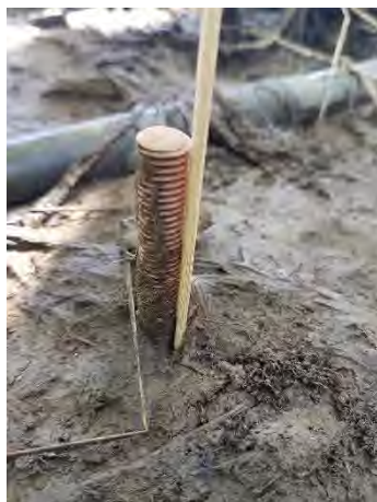
Figure 42: Image capture of erosion pegs following completion of the plant crop harvest. The level of deposition was recorded by measuring the distance between the washer and soil surface (using a skewer)
