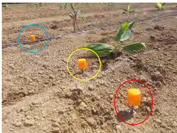
Figure 40: Three erosion pegs were installed on the southern side of each ground cover treatment and replicate. One peg near the irrigation line (highlighted blue), one in the middle of the southern side (yellow) and another peg installed on the outside shoulder of the bed (highlighted in red)
