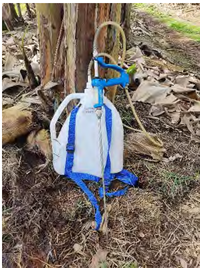
Figure 9: Knapsack and injecting gun used to apply the EPN treatment
