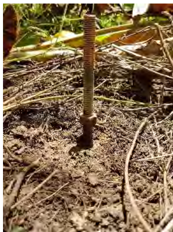
Figure 41: Image capture of erosion pegs following completion of the plant crop harvest. The amount of erosion was recorded by measuring the distance between the washer and nut
