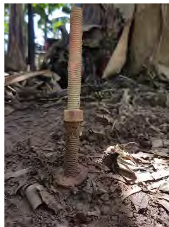
Figure 41: Image capture of erosion pegs following completion of the plant crop harvest. The amount of erosion was recorded by measuring the distance between the washer and nut
