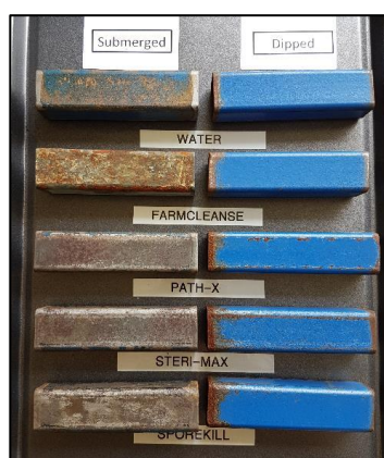
Figure 7: Painted steel, submerged in solution (left), dipped frequently (right)
