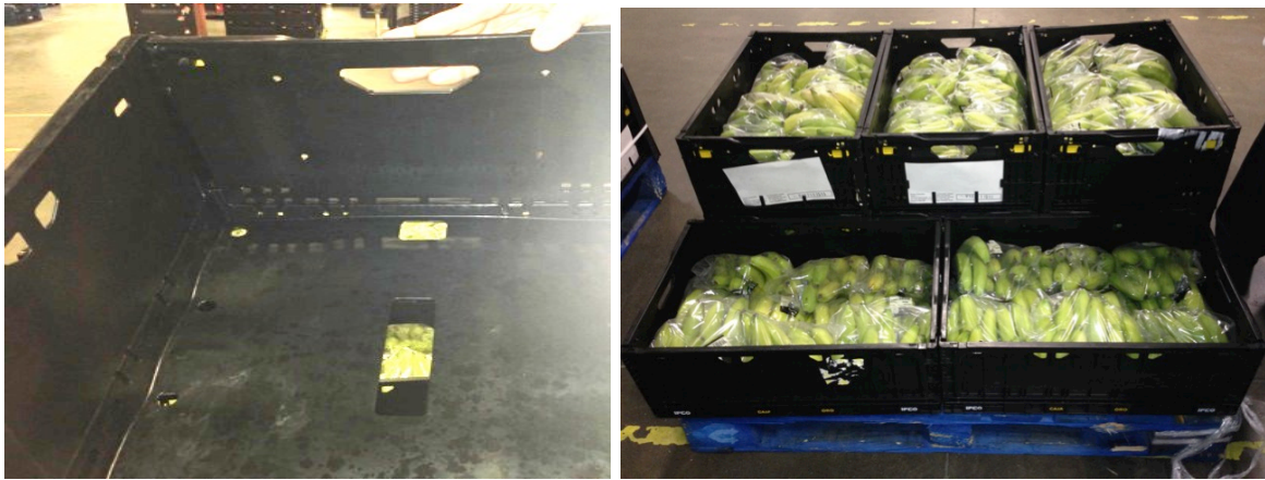
Figure 24 and 25: RPC used by ASDA to transport bananas direct to stores from the tropics (note the smooth internal faces)
