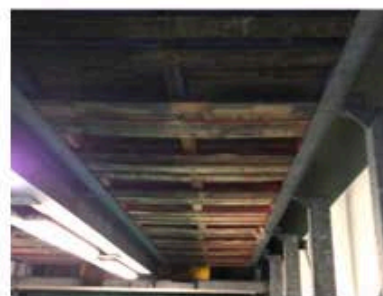
Figure 12: Bowing pallets in leading to compression of fruit
