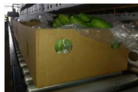
Figure 13 & 14: Fruit packed proud in the carton is prone to compression bruising, albeit some settling will occur
