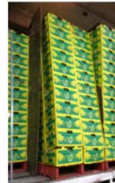
Figure 9 & 10: Lack of support during transit allows pallets to become unstable
