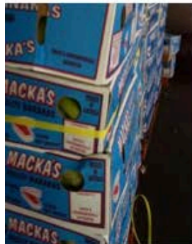
Figure 5 & 6: Over-tensioned pallets causing cartons to collapse
