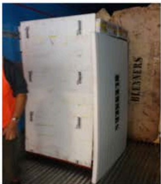
Figure 23 & 24: Foam padding and plywood sheets used to help stabilize pallets and prevent movement during transit
