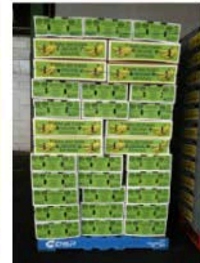
Figure 9 & 10: Lack of support during transit allows pallets to become unstable
