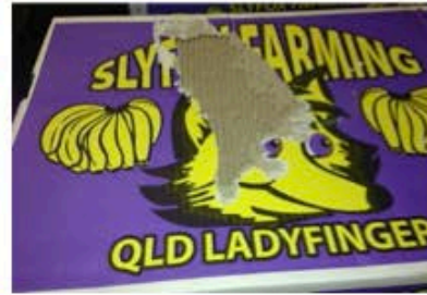
Figure 1 & 2: Excessive and incorrect glue creating increased 'breaking strain' when cartons are separated causing cartons to tear
