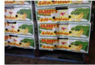
Figure 4: Forklift trucks without 'pallet pickers' can damage cartons
