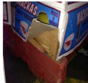
Figure 7 & 8: Damaged pallets and pallets with planks spaced too far apart cause damage to bottom layer cartons
