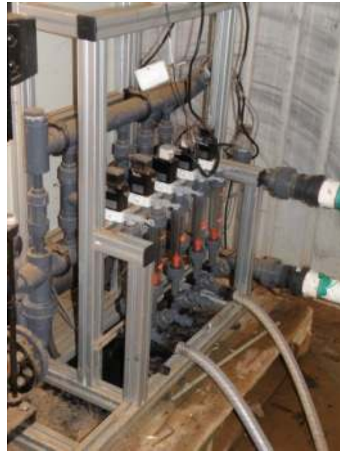
Fertiliser dosing channels working through the irrigation controller. Photo: DAFWA
