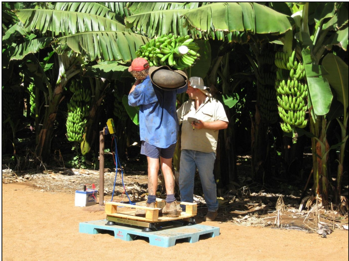
Figure 2. Walk-over weigh system used for collecting bunch weights. Net weight of the bunch was calculated from gross weight less the pickers' body weight.
