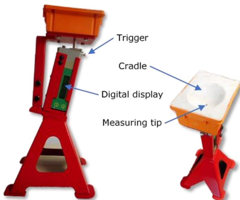
**Figure 2.** Prototype bench-top configuration of FruitFirm Meter for avocado fruit firmness assessment.
