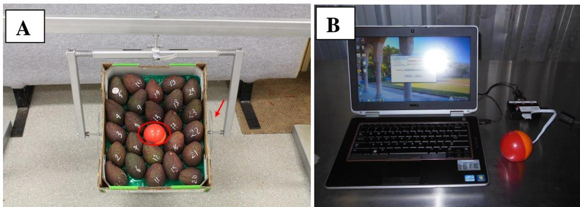
**Fig. 2.3** A: Arrangement of avocado cv. 'Hass' fruit in a tray held in the avocado tray drop equipment for drop from treatment specific height and drop angle. The red circle highlights the impact recording device placed in the center of the fruit tray. The red arrow points to a protector fitted to help adjust drop angles. B: The IRD connected with the laptop for set up for data acquisition or for data downloading.
