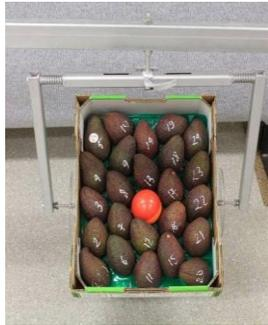
Impact recording device and shock loggers were used in these experiments for their calibration for further use in the supply chain studies.
