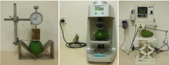
Measurement of fruit firmness with analogue firmness meter (Left), SIQ firmness tester (Middle), and electronic firmometer (Right)
