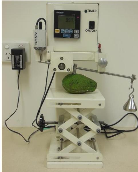
**Fig. 2.5** Anderson® Electronic Firmometer. A 9 mm diameter probe contacts the fruit under a load of 200g applied on a lever arm for 10 sec. The objective value of firmness is displayed (mm).
