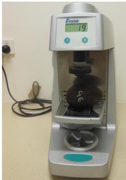
**Fig. 2.4** The Sinclair Internal Quality Firmness Tester. A piezoelectric sensor at the tip of the air-blow bellows taps at four points around the horizontal axis of the fruit and the liquid crystal
