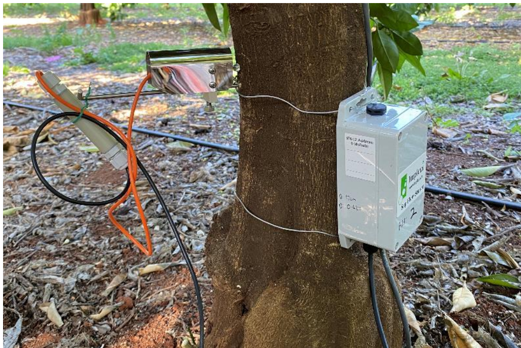
Figure 5. SAP flow and trunk dendrometer installed on a navel tree.
