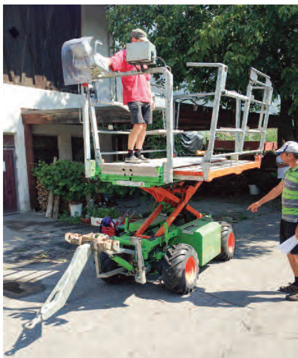
Samotec EVO4: A powerful electric driven platform quietly handles steep terrain, bins, has ultrasonic sensors for steering and electromagnetic energy recovery (i.e. recharges downhill). Photo shows Martin Thommann from Beratungsring on the right.
