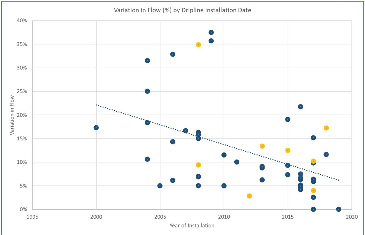
Figure 2 Relationship between dripline age and variation in flow rate (blue circles are sites with pressure compensating emitters, yellow circles have non-pressure compensating emitters)
