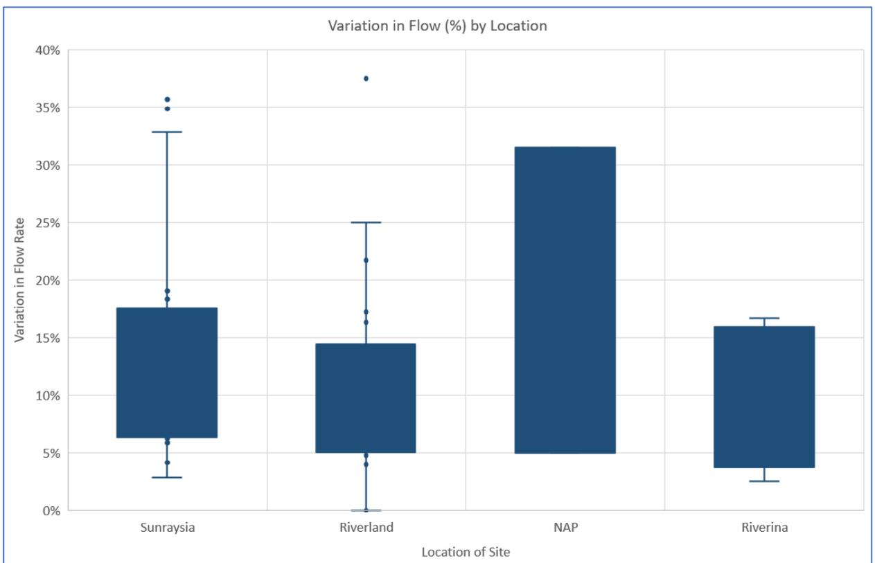
Figure 3 Relationship between orchard location and variation in flow rate
