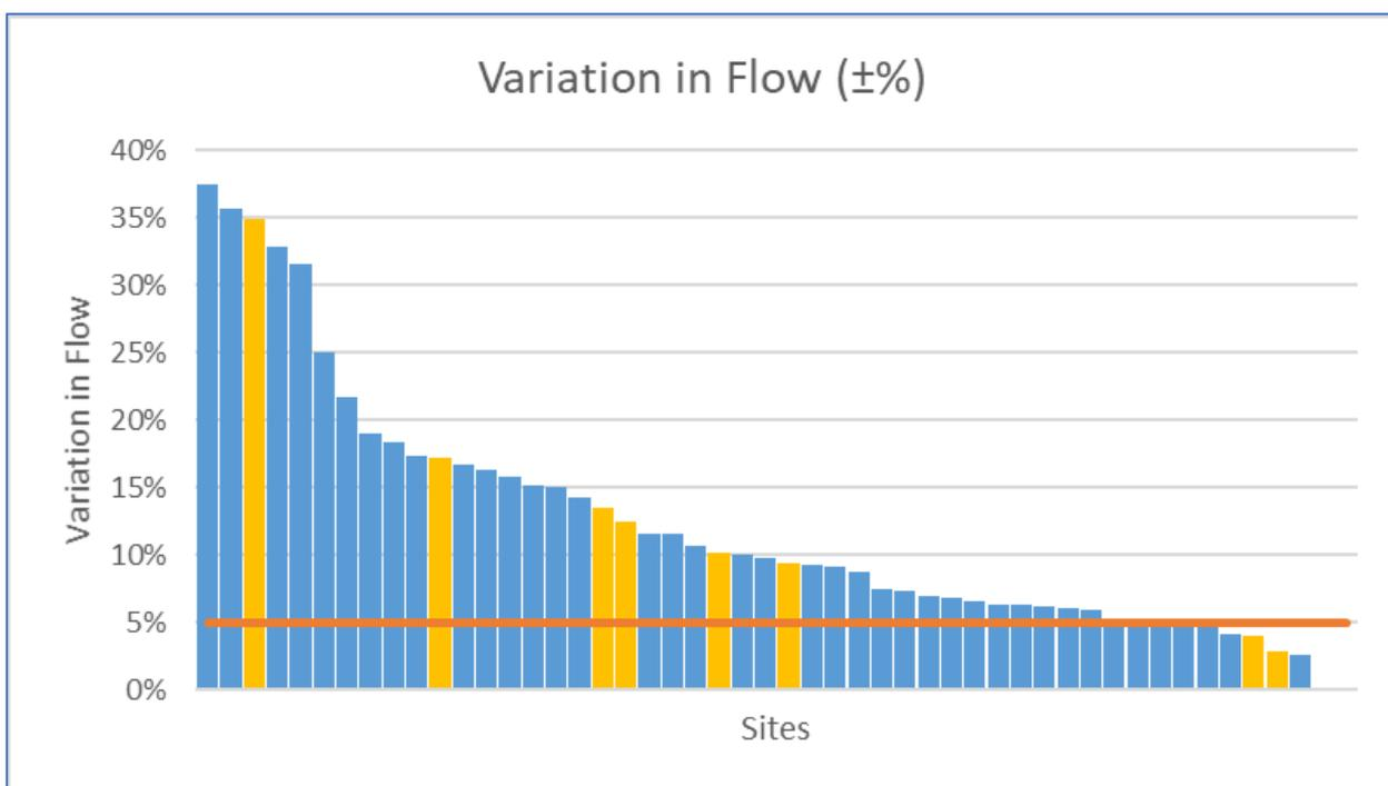
Figure 1 Sites ranked by variation in flow rate, standard = <5% (blue bars are sites with pressure compensating emitters, yellow bars have non-pressure compensating emitters)
