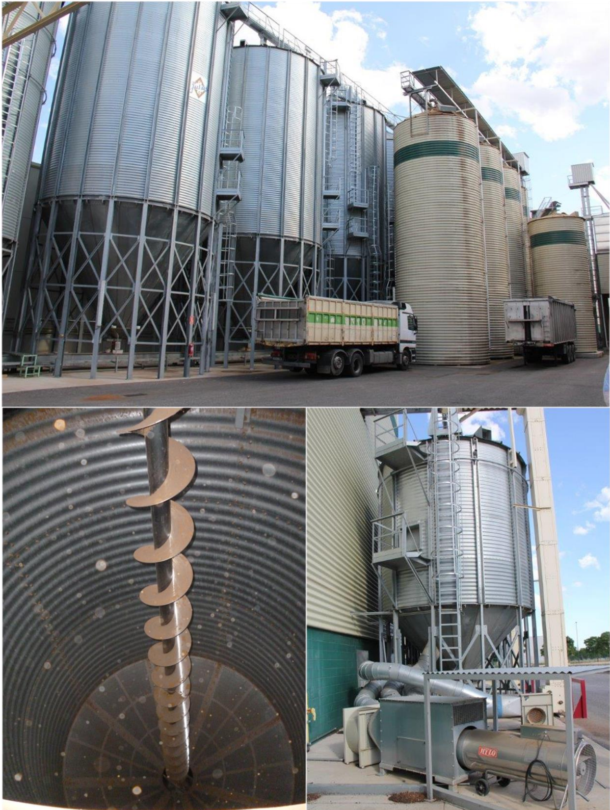
Figure 7: Almond silos (top), drying silo with auger (bottom left) and drying silos (bottom right)
