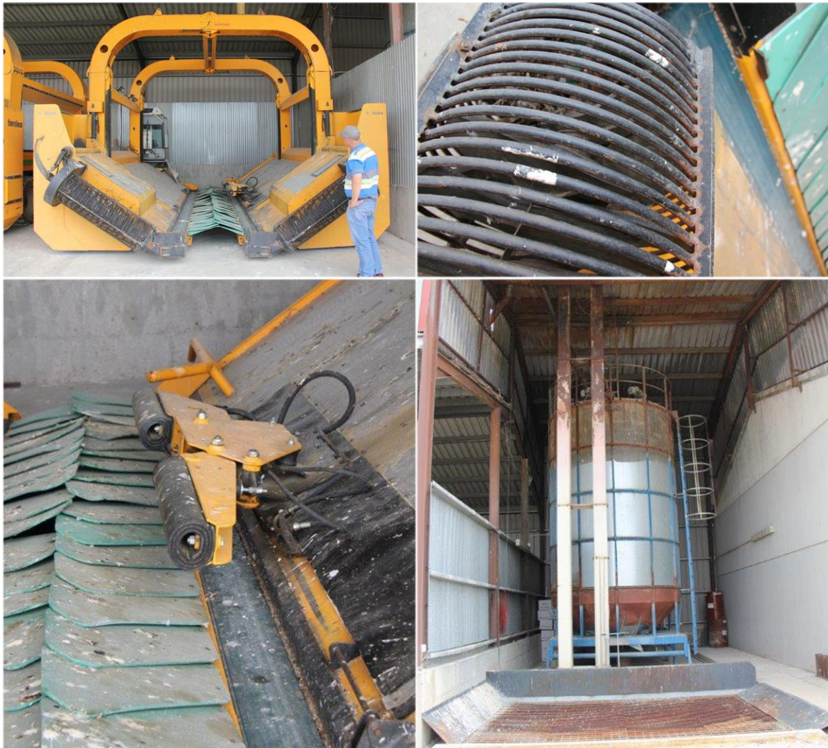
Figure 6: Tenias over the row shake and catch harvester, in-field de-huller, silo for drying in-shell crop, and shaking head (clockwise from top left)
