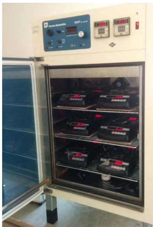
Figure 3. Controlled dehydration using data logged scales being undertaken with temperature and humidity control
