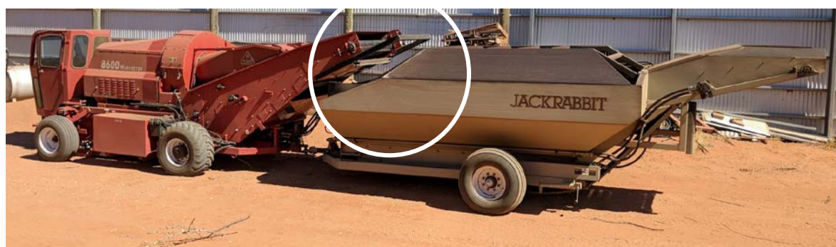
Figure 22. Yield mapping system fitted between harvester and surge cart (circled)
