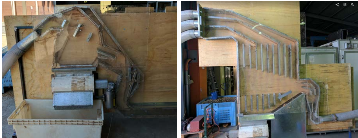
Figure 19. Several of the iterations toward the design of a detached hull separator
