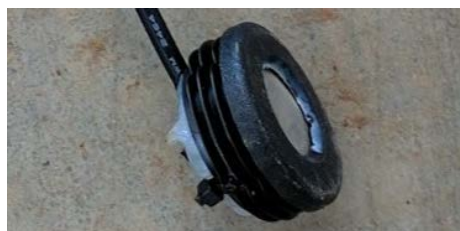
Figure 8. A temperature and humidity sensor in a mounting plug
