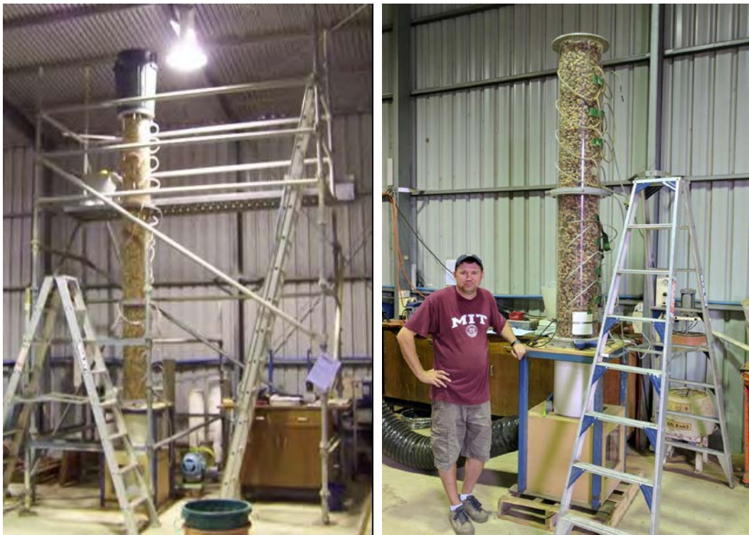
Figure 1. Michael Coates with his instrumented 3m and 2 m drying tower
