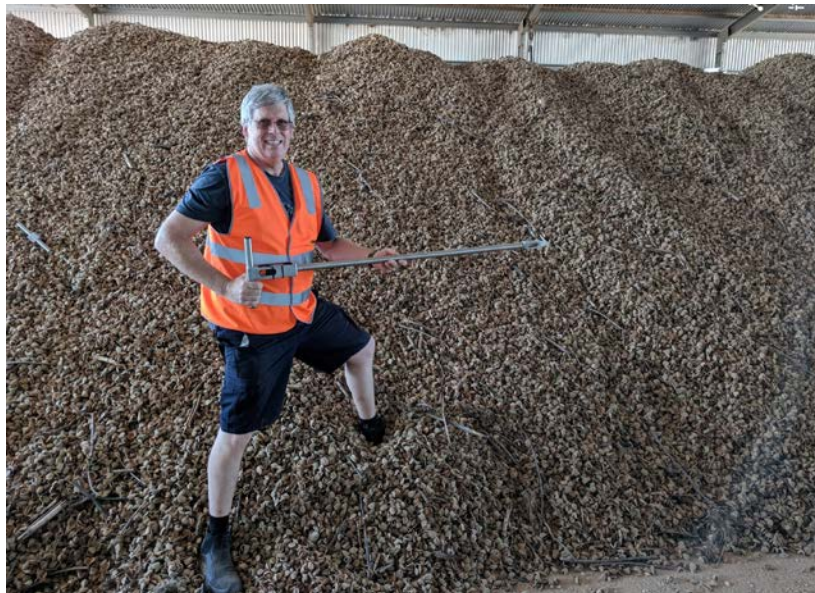
Figure 12. Commercial temperature and humidity sensor (top) and Professor John Fielke with it mounted into a spear (bottom)
