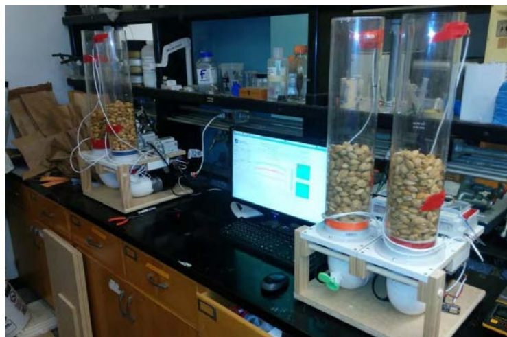
Figure 2. Laboratory scale dryers used in Australia and California
