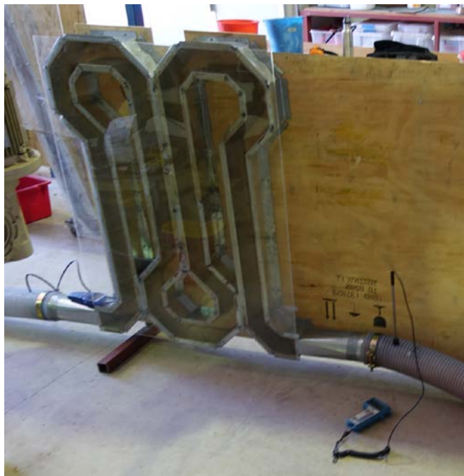
Figure 16. Prototype huller with clear face to observe performance
