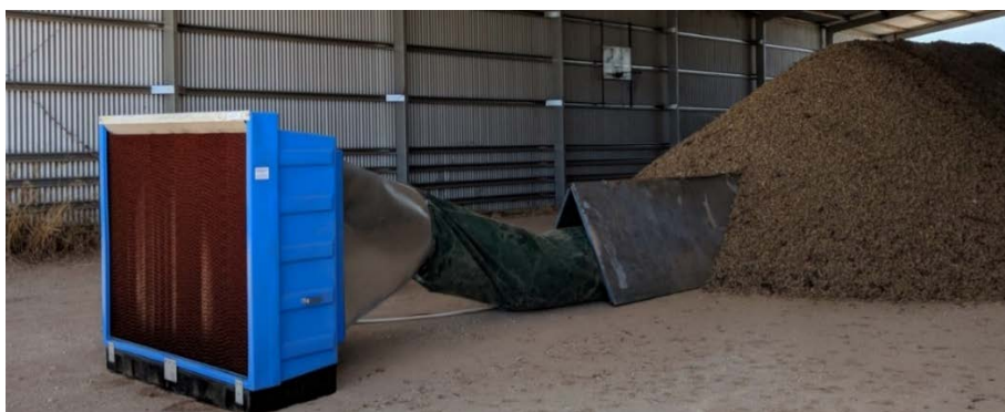
Figure 9. QC48 Evaporative cooler fitted to the aeration duct. Select Harvests' Allinga Farm
