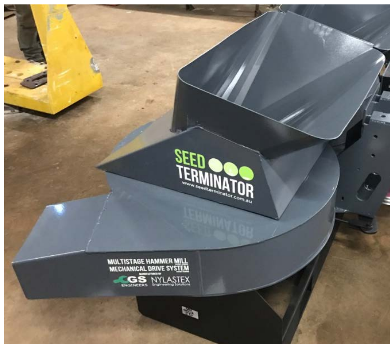
Figure 35. Seed Terminator multi-stage hammer mill ( https://twitter.com/seed_terminator/status/910852788145369088 )
