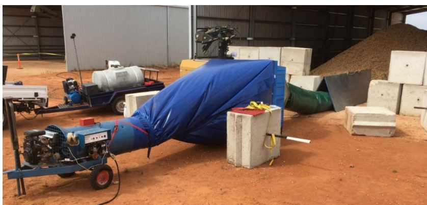
Figure 10. Additional fan added to evaporative cooler. Select Harvests' Allinga Farm
