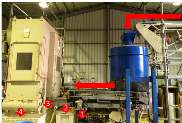
Figure 14. Impact thresher and screen separator used to process almonds with four outputs for (1) small pieces of shell and hull, (2) kernel, (3) in-shell and in-hulls passing over the screen and (4) light waste separated by air cleaner
