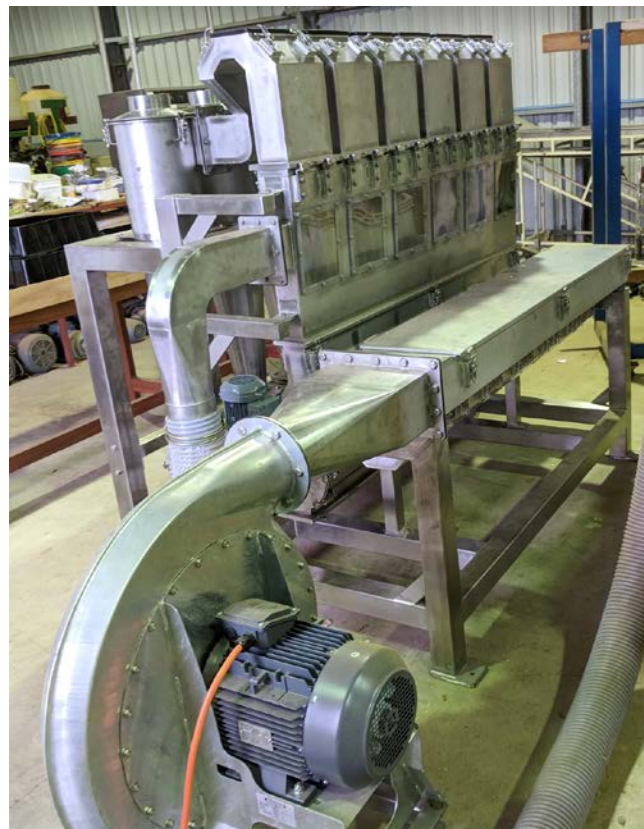
Figure 20. Final design of the detached hull separator
