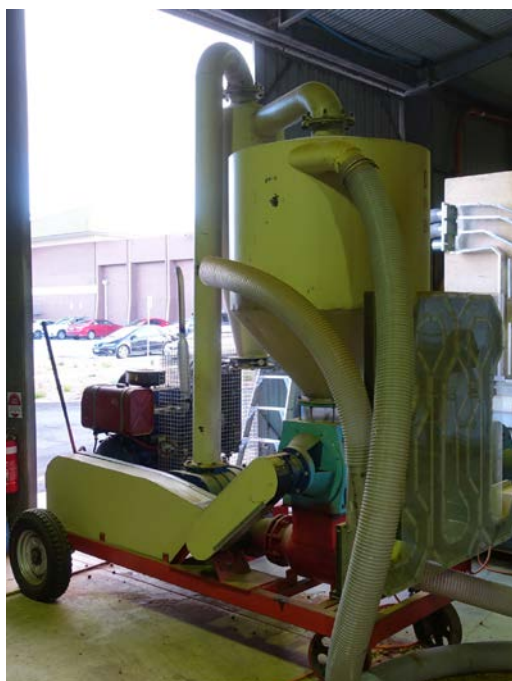
Figure 17. Pneumatic conveyor used to convey the almonds through the huller and separator
