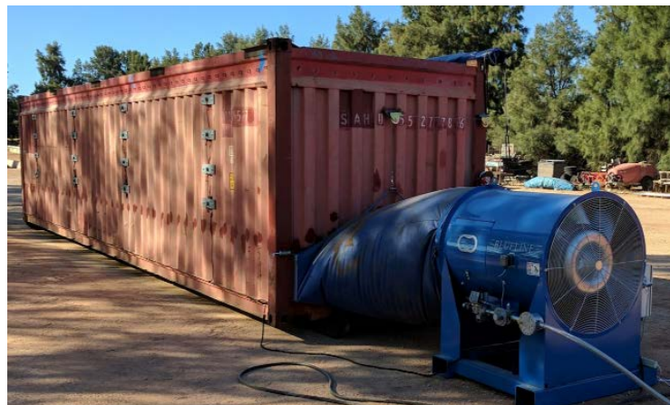
Figure 6. 40' shipping container used for drying of rain affected re-shake almonds at Jubilee Almonds
