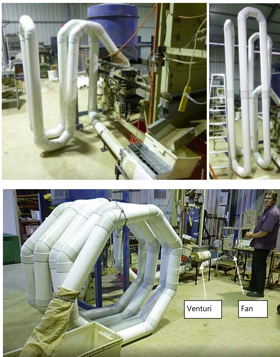
Figure 15. Various arrangements for impact hulling and shelling using a PVC pipe with venturi infeed
