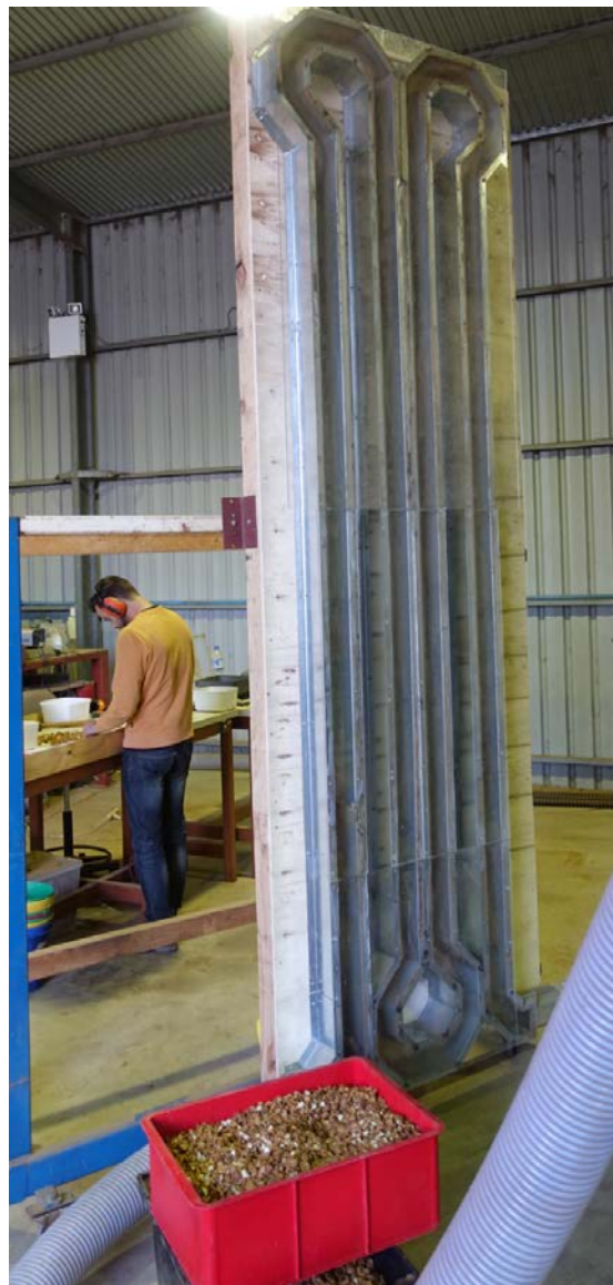
Figure 21. 3m high impact sheller for hard shelled almonds
