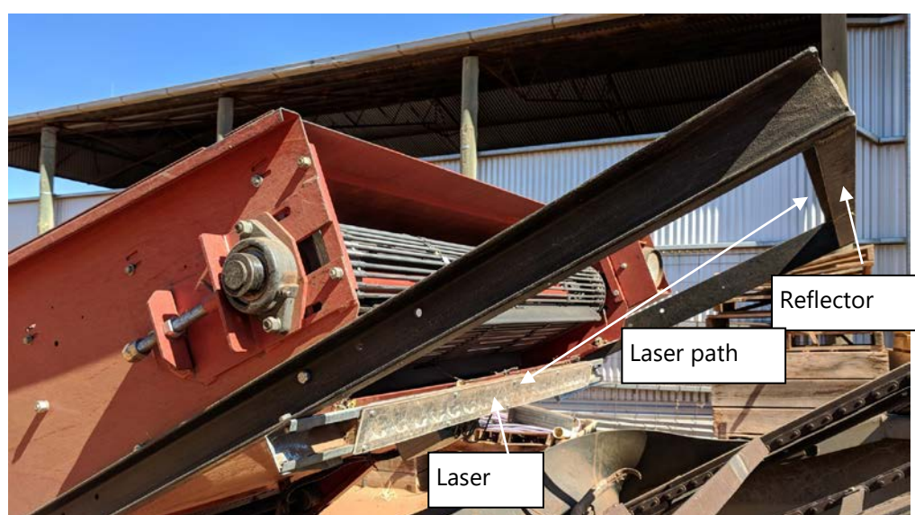
Figure 23. Details of yield mapping system fitted between harvester and surge cart
