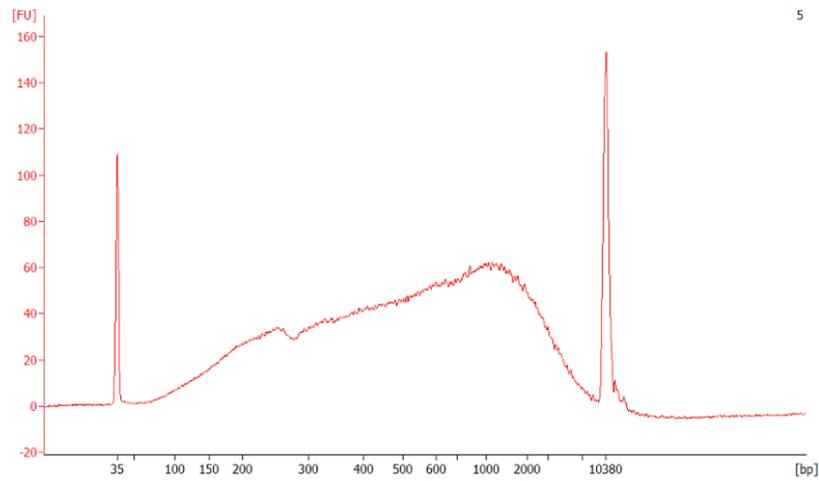
The figure shows poor shearing when followed the protocol developed for model species
