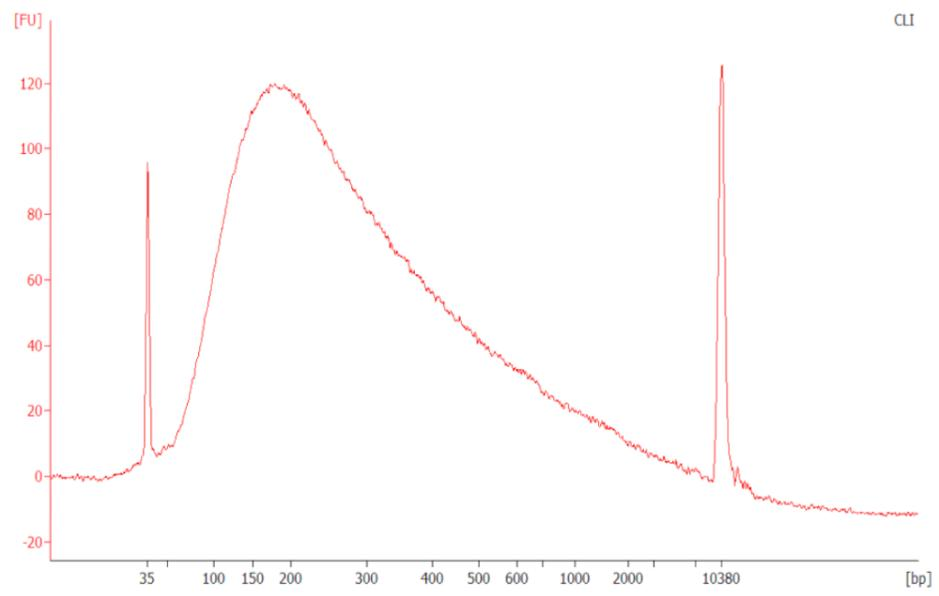
Fig 1. An example of product size after sonication using Bioruptor at 30 sec on, 30 sec off at high speed for 70 - 80 minutes
