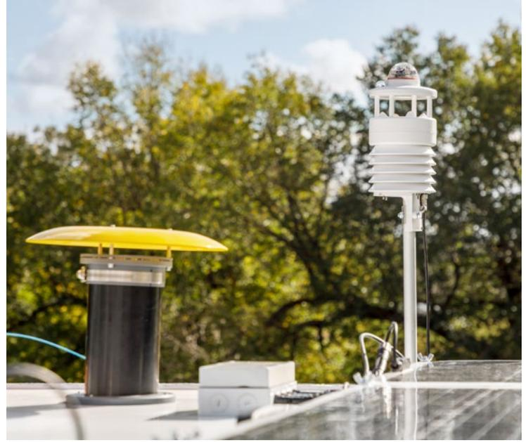
Sentinel trapping devices including the two-metre insect trap, spore sampler, and weather station.
