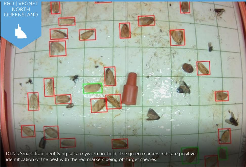
DTN's Smart Trap identifying fall armyworm in-field. The green markers indicate positive identification of the pest with the red markers being off target species.
