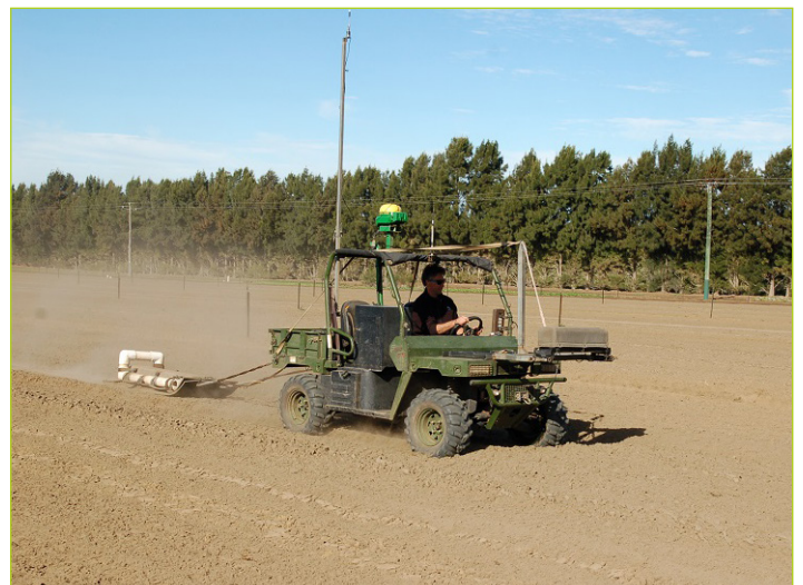
Figure 8. EM and radiometric soil mapping in action. Note radiometric sensor on the front of the vehicle. Source: Vegetables WA
