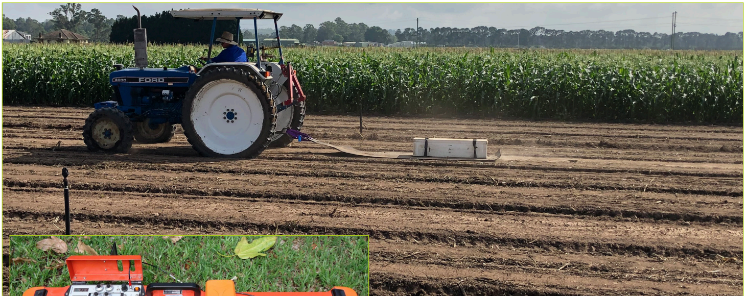
Figure 2. EM38 sensor (close-up inset) being towed behind a tractor to map soil electrical conductivity variability across a mixed vegetable farm in NSW. Source: Precision Pastures
