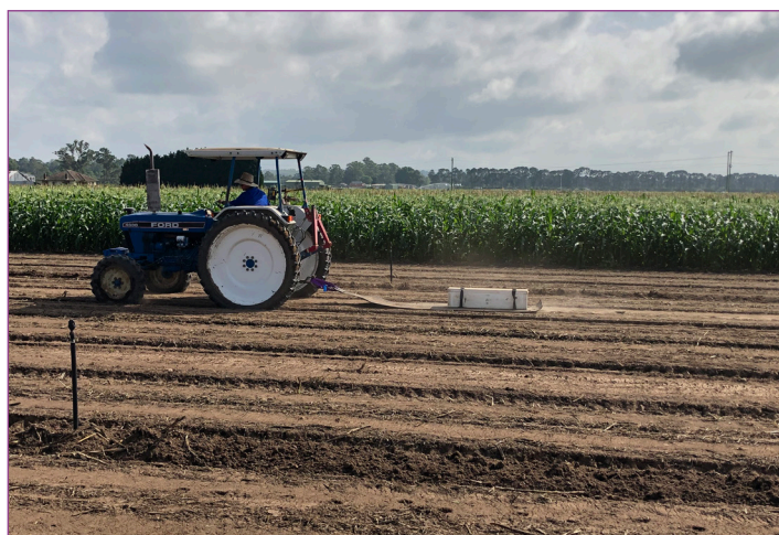
Figure 1. EM38 sensor (top) being towed behind a tractor (lower) to measure soil texture at different points in the field. Source: Precision Pastures.
