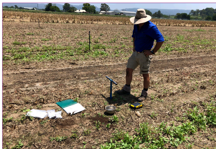
Figure 3. Soil sampling was conducted at each of the zones identified by the EM38 map. Source: Precision Pastures.
