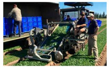
**Photo 1.** Harvesting babyleaf spinach with a purpose-built harvester.
